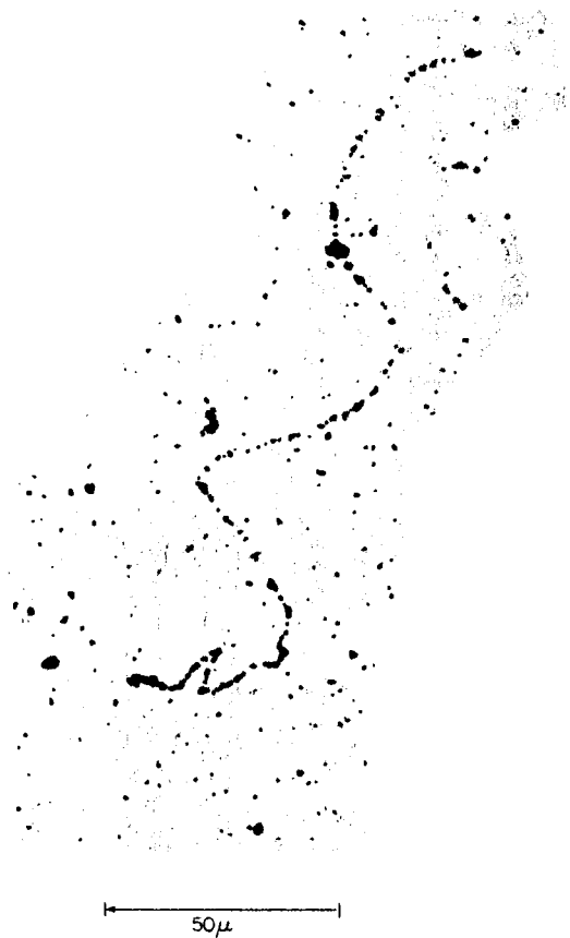
Figure 5-4. Photomicrograph of approximately 300-keV electron track in a nuclear track emulsion. (7c)
