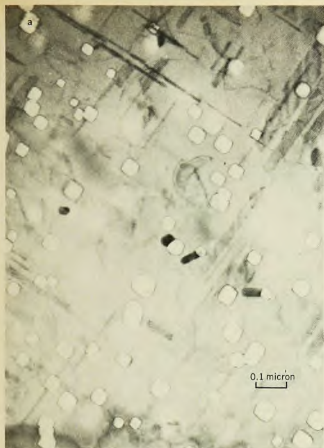
Voids produced by bombardment with 7.5-MeV tantalum ions. In vanadium (a), bombardment at 700 deg C has caused about 30 displacements per atom, while the niobium in b was bombarded to 300
