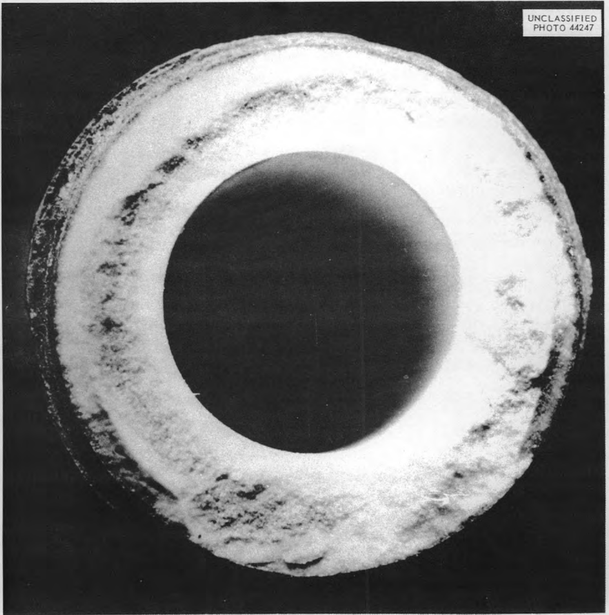
Fig. 3.2. Fractured Surface of Alumina Tube.
