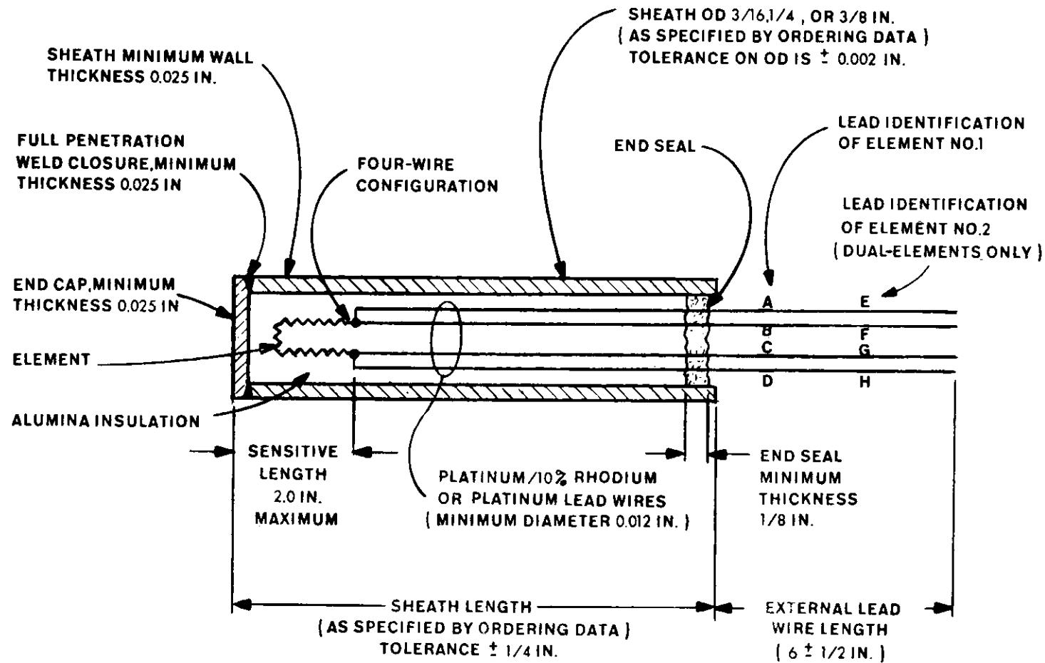
Fig. 1. Thermometer Construction Features and Standard Dimension Requirements.
