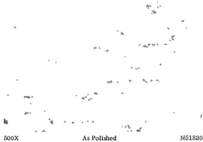
FIGURE 9. CHROMITE IN LOW-SILICON PREALLOYED TYPE 318 STAINLESS STEEL DUE TO OXYGEN CONTAMINATION OF THE POWDER DURING THE SHOTTING PROCESS
