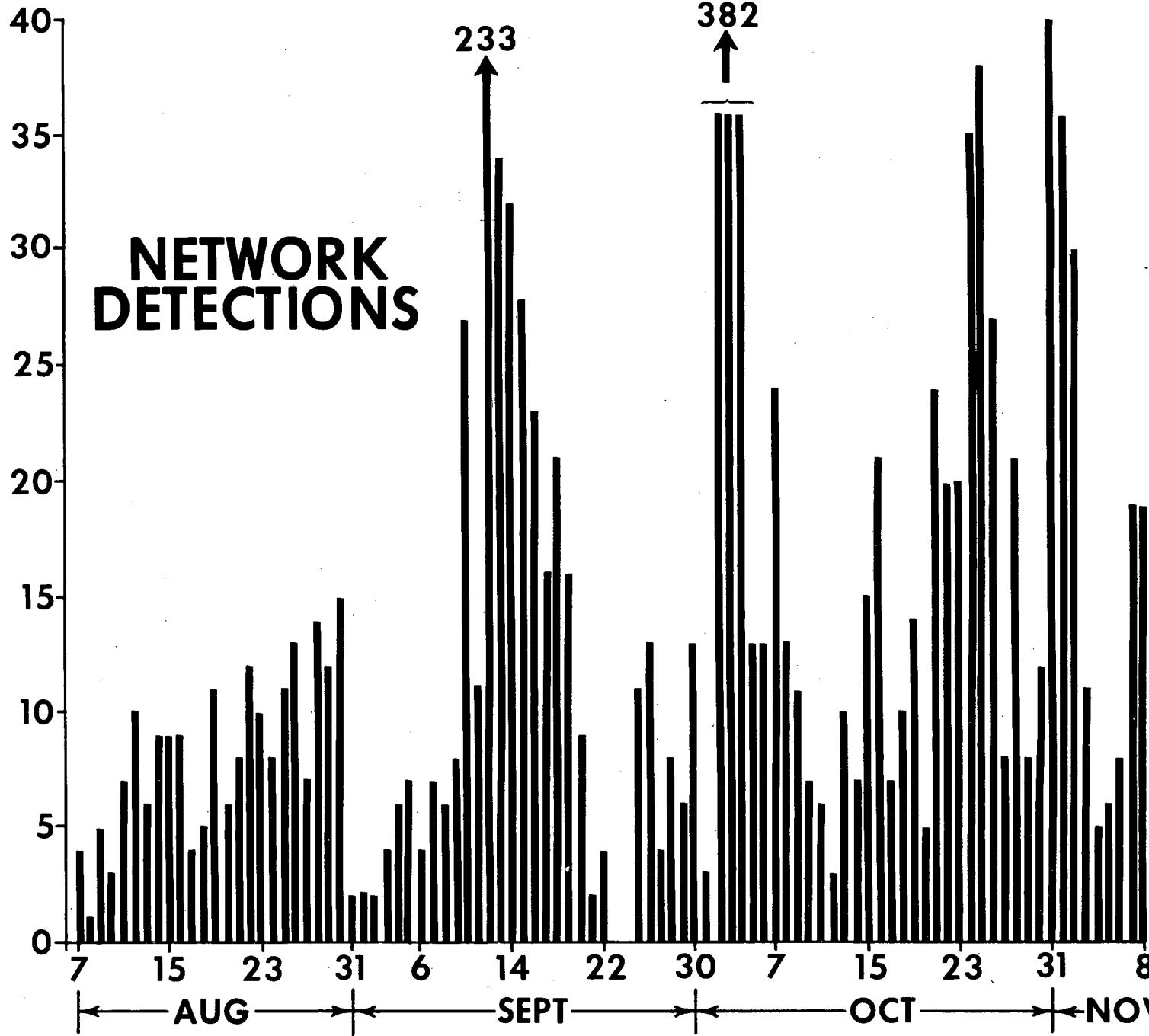
This distribution shown also reflects, of course, the variable capability of the network due to weather conditions and operational data dropout. The 382 events following MILROW are predominantly aftershocks of the type previously discussed. Outside this phenomenon, there is little in the frequency of natural earthquake activity following MILROW to distinguish it from the pre-MILROW monitoring.
