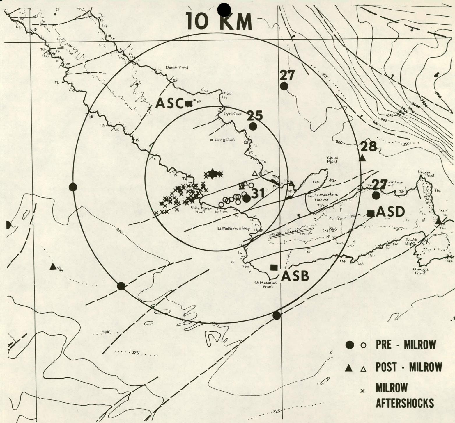
may be related to movements along major tectonic blocks in close proximity to ground zero. The epicenters and focal depths of earthquakes in this category are shown in Figure 8 by solid circles and triangles. The focal depths are remarkably similar and indicate movements along a fault very close to 28 km under Amchitka. That this depth constitutes the location of a major thrust fault passing under the ridge at this point is highly likely.
