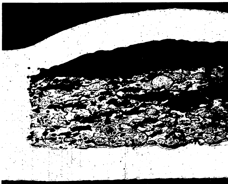
Fig. II-25 Typical core cross section of a sample fuel plate after failure has occurred by blistering.
