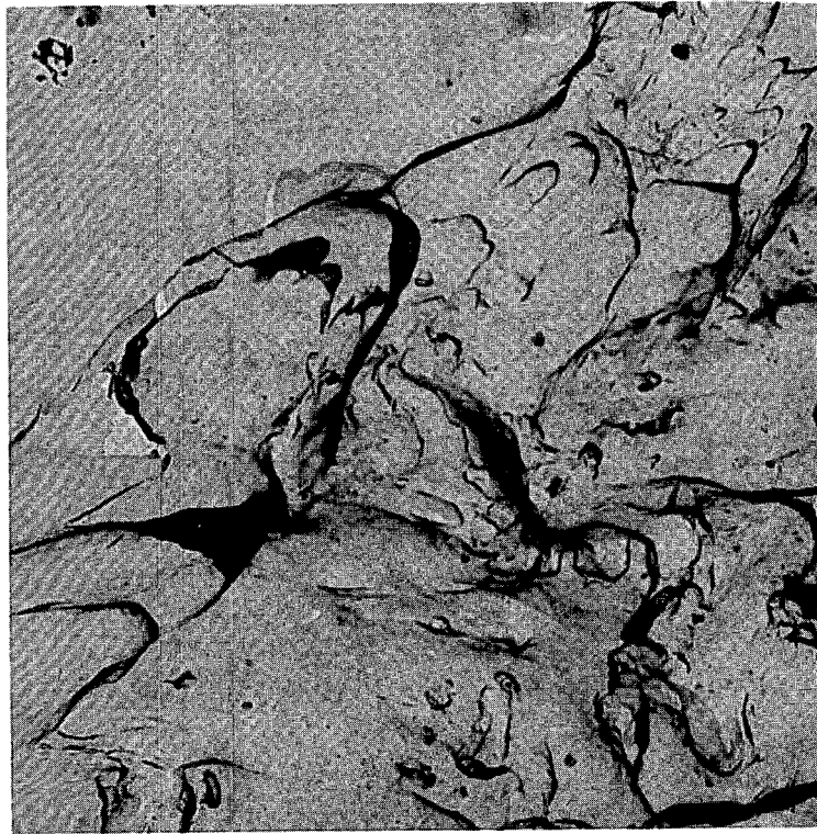
Fig. II-32 Ductile structure of fractured air line showing dimpling.
