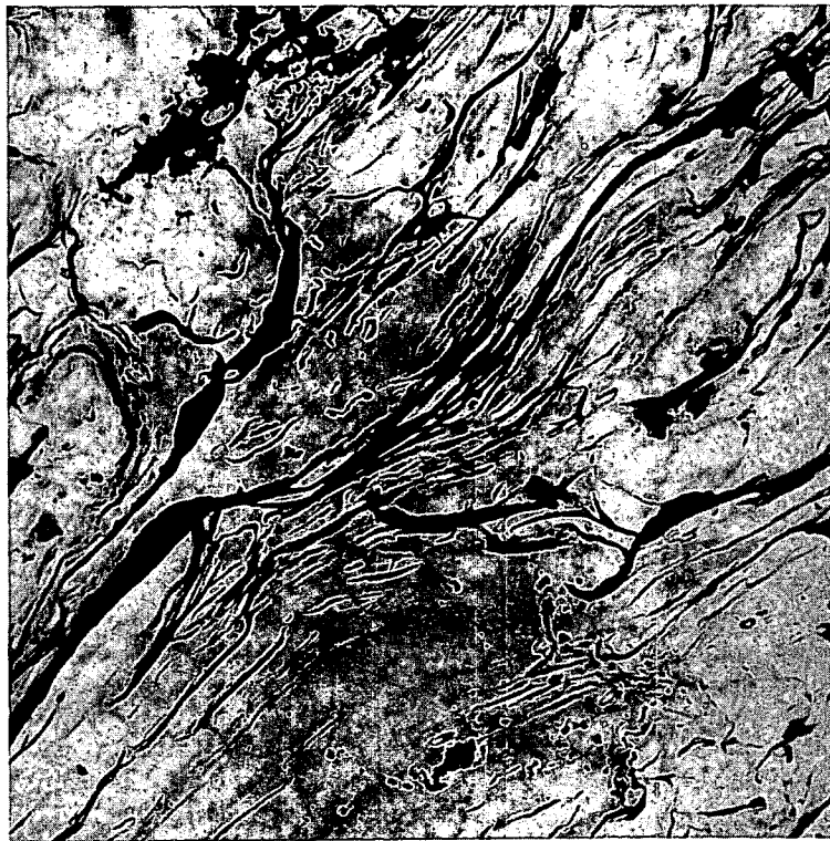
Fig. II-34 "River" structure from fractured air line indicating brittle behavior and a running crack. This is from opposite the breakover point area.
