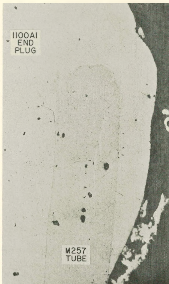
Figure 7. Fusion Welded End Closure of 1100 Al End Plug in M257 Tube
