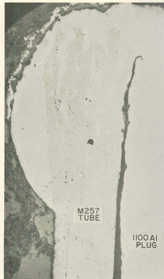
Figure 8. Fusion Welded Joint of 1100 Al and M257, Showing Segregation of Oxide Induced by Overheating
