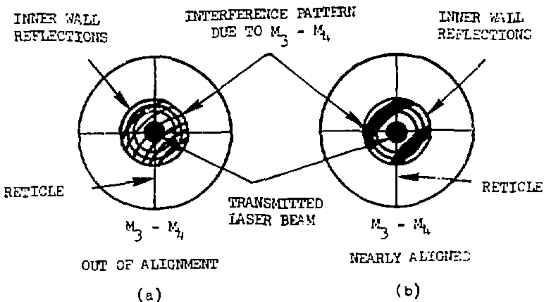
Figure 5. Interference Fringes Due to  $M_3$ - $M_4$  Misalignment
