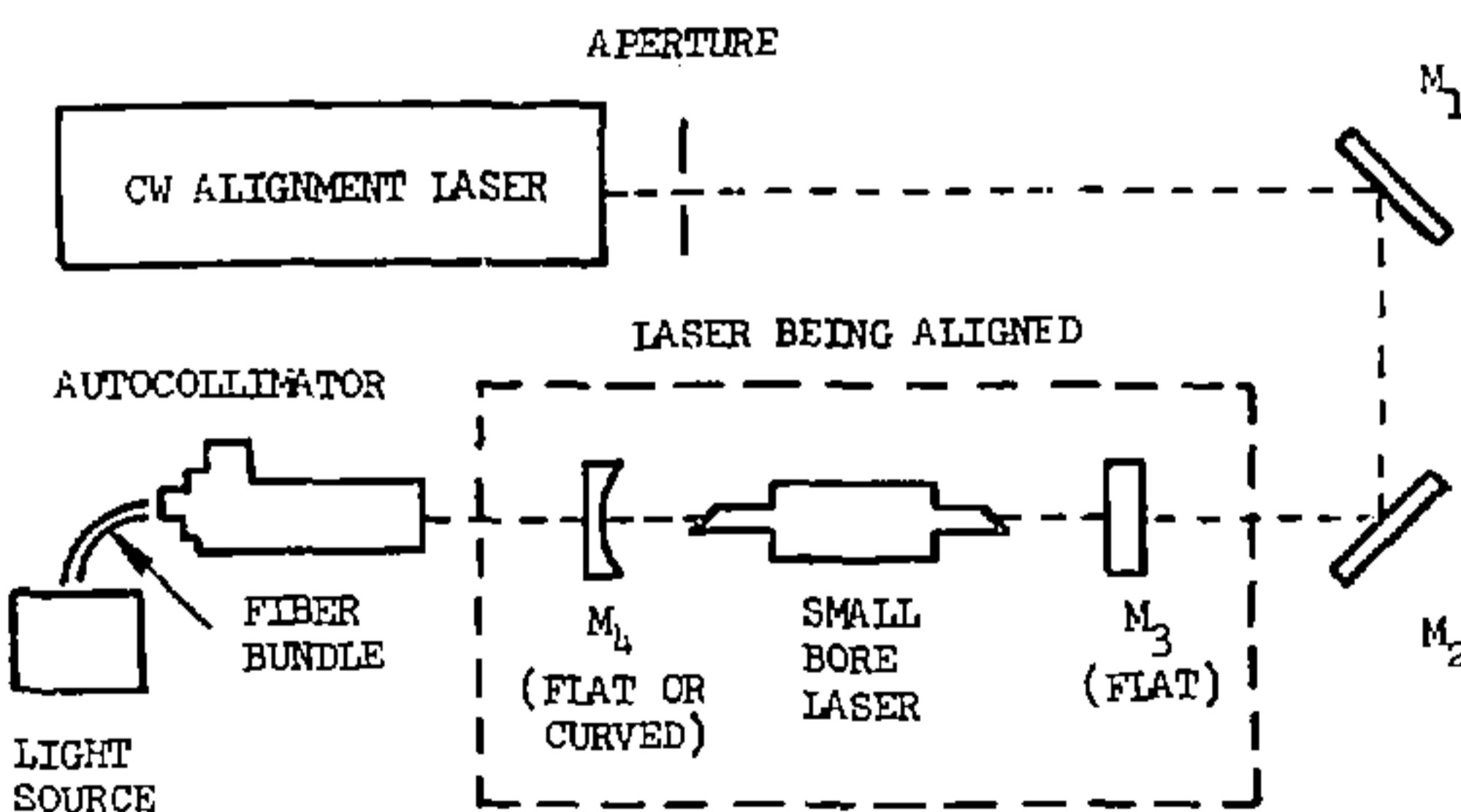
Figure 1. Alignment Set Up
