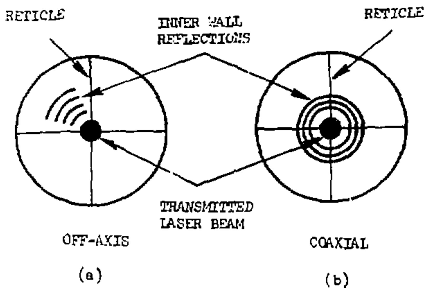
Figure 1. Pattern Observed in Autocollimator
