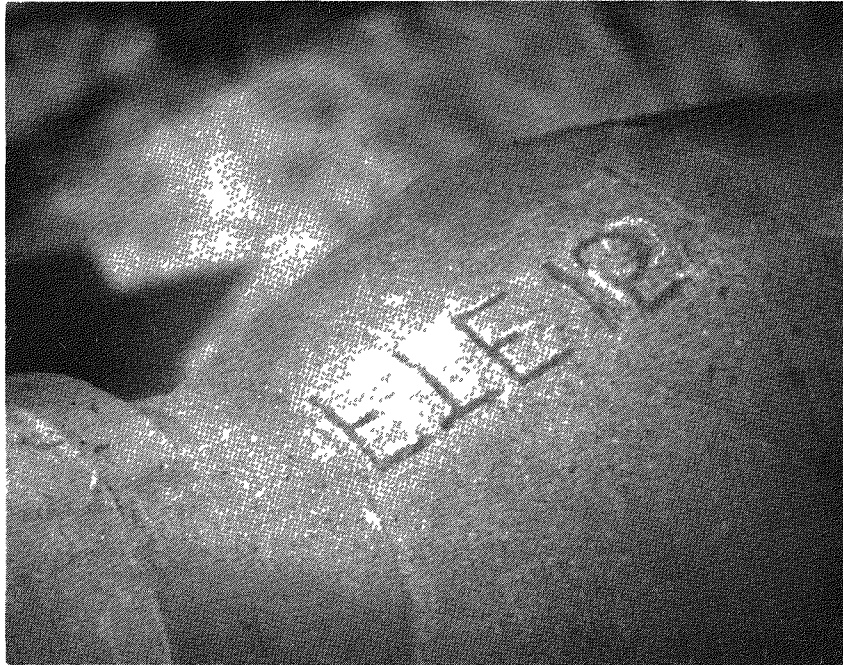
Fig. 9-64. Fuel test element identification, FTE-15 (mirror image)
