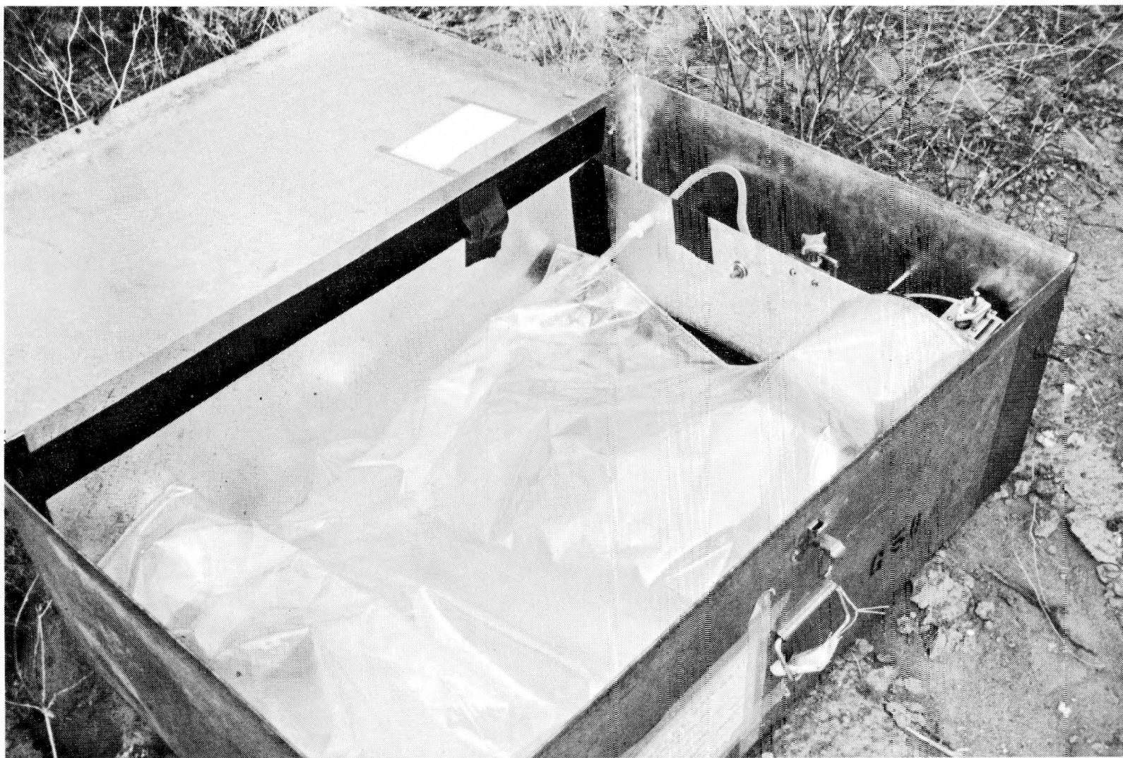
Figure 4. Example sampler used to fill saran bags at the fixed ground-level positions. The sampler pump is seen at the upper right corner of the box.
