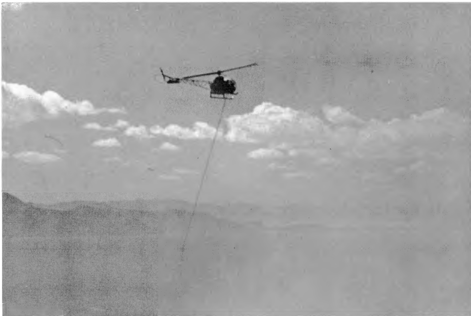
Figure 5. . Sampling helicopter enroute to the next sampling position. The sampling inlet is at the bottom of the hose shown below the helicopter.
