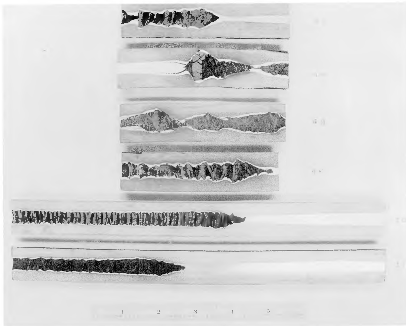
Fig. 7 - Longitudinal sections of Design I, extrusions 21447, 21448, 21449, 21446, 21930 and 21931, reading top to bottom. The centrally-located UO_2 is separated by stainless steel from the cold-rolled steel shell. Nital etch. Extrusion 21930 provides a good example of "wafering". Extrusion direction is from left to right. RF-7224.
