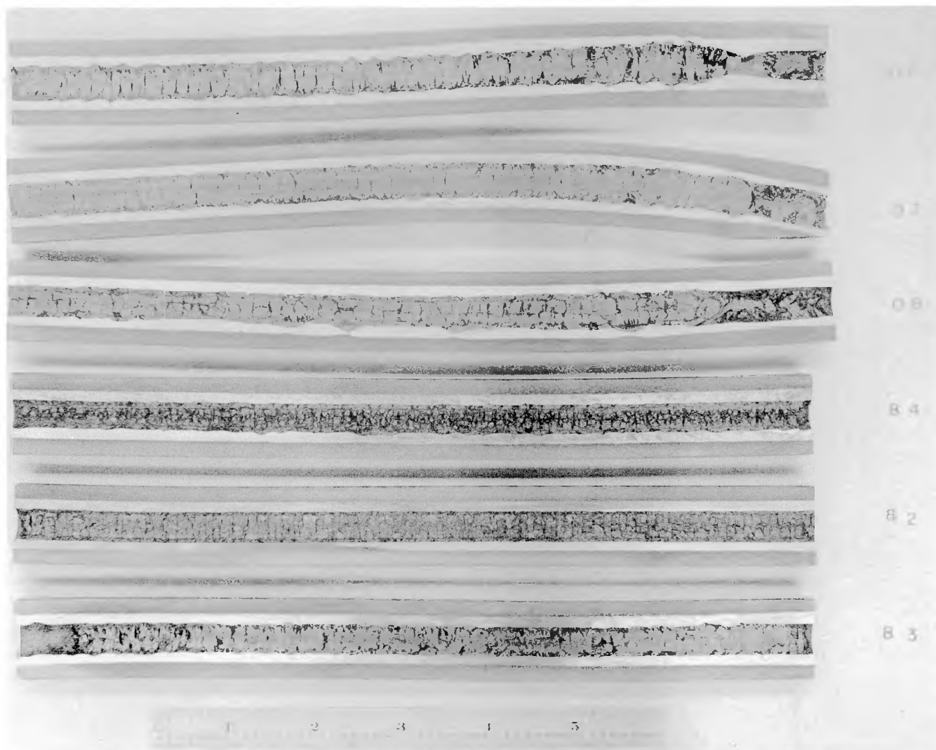
Fig. 10 - Longitudinal sections of Design V coextrusions, 21806, 21807, 21808, 21884, 21882 and 21883, reading from top to bottom. Nital etch. The UO_2 in the middle is bounded in succession by extruded graphite, stainless steel and cold-rolled steel. Scattered remnants of 0.003-inch tantalum foil bound the UO_2 for extrusions 21806, 21807, 21808 and 21884. Extrusion direction is from left to right. RF-7226.
