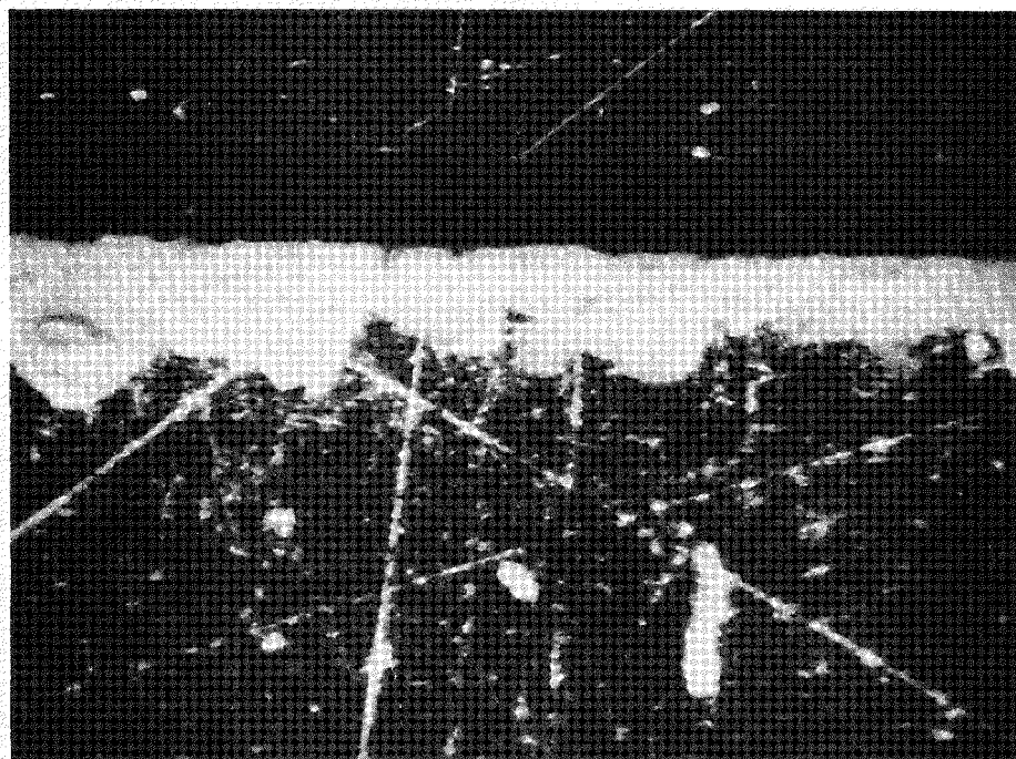
Exhibit B - Aluminum 1100 exposed to fluorine at 1020°F for 24 hours.
