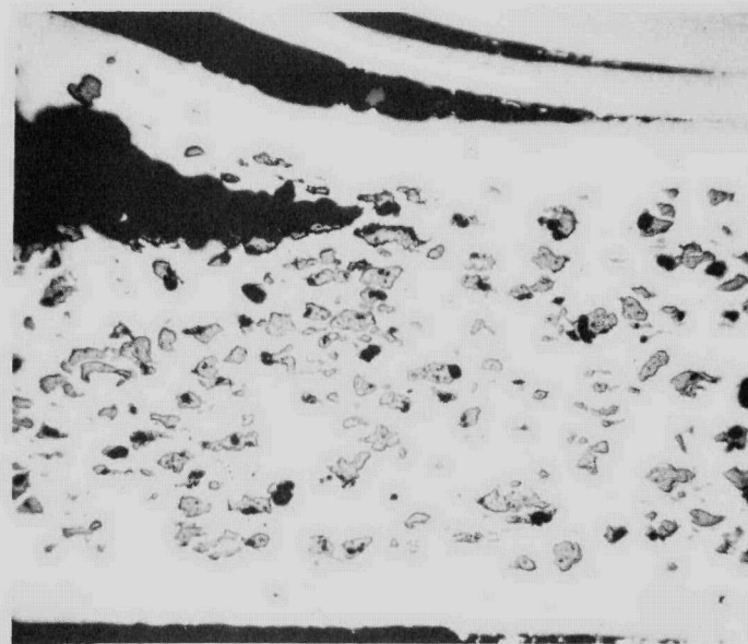
FIGURE 19. AREA UNDER BLISTER ON SPECIMEN 55
