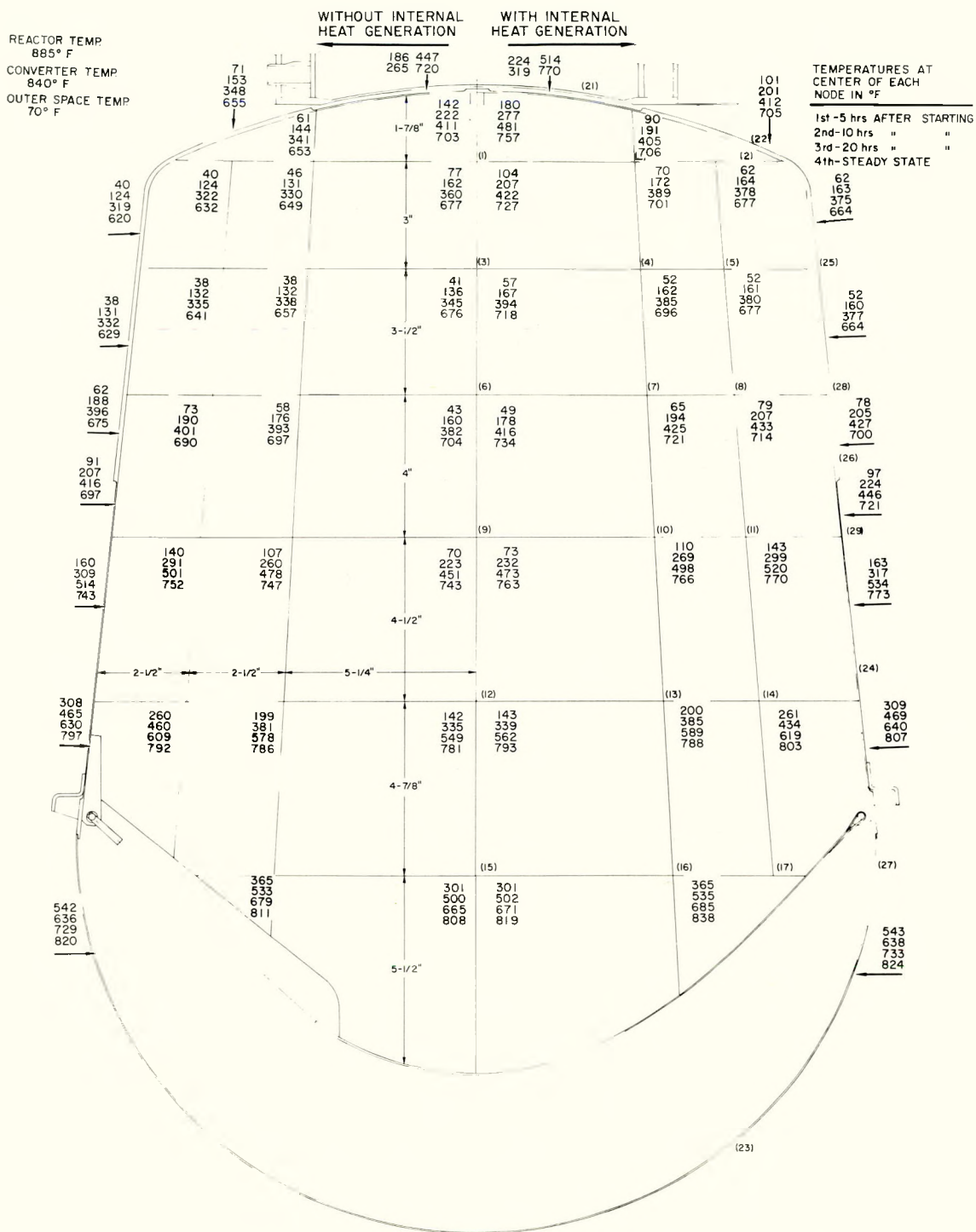
Figure 11. SNAP 10A Shield Temperatures (LiH in Pressed Form)
