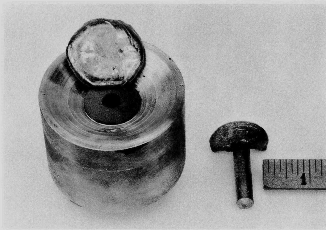
FIGURE 1. ASSEMBLED MOLD WITH ARC-MELTED UC BUTTON CHARGE AND FINISHED CASTING
