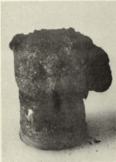
Experiment No. 7 Hastelloy C Temp. (T.C.) >2500°F
