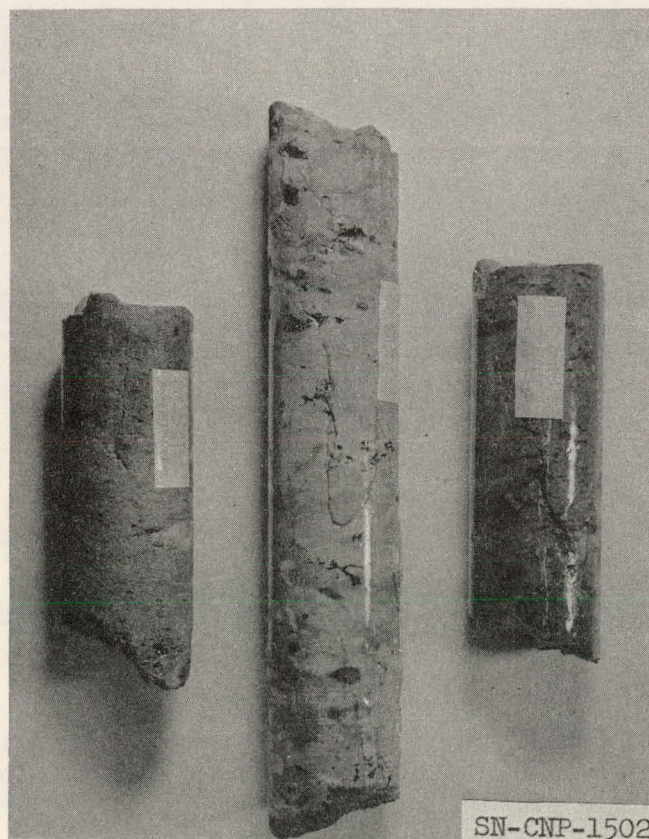
Fig. 8. Primary (blast) tension fractures in core from U12-B Rainier hole H.
