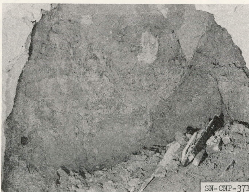
Fig.6. Pulverized rock (TOS 7-7r ) in central collapse block U12-B Exploratory Drift.
