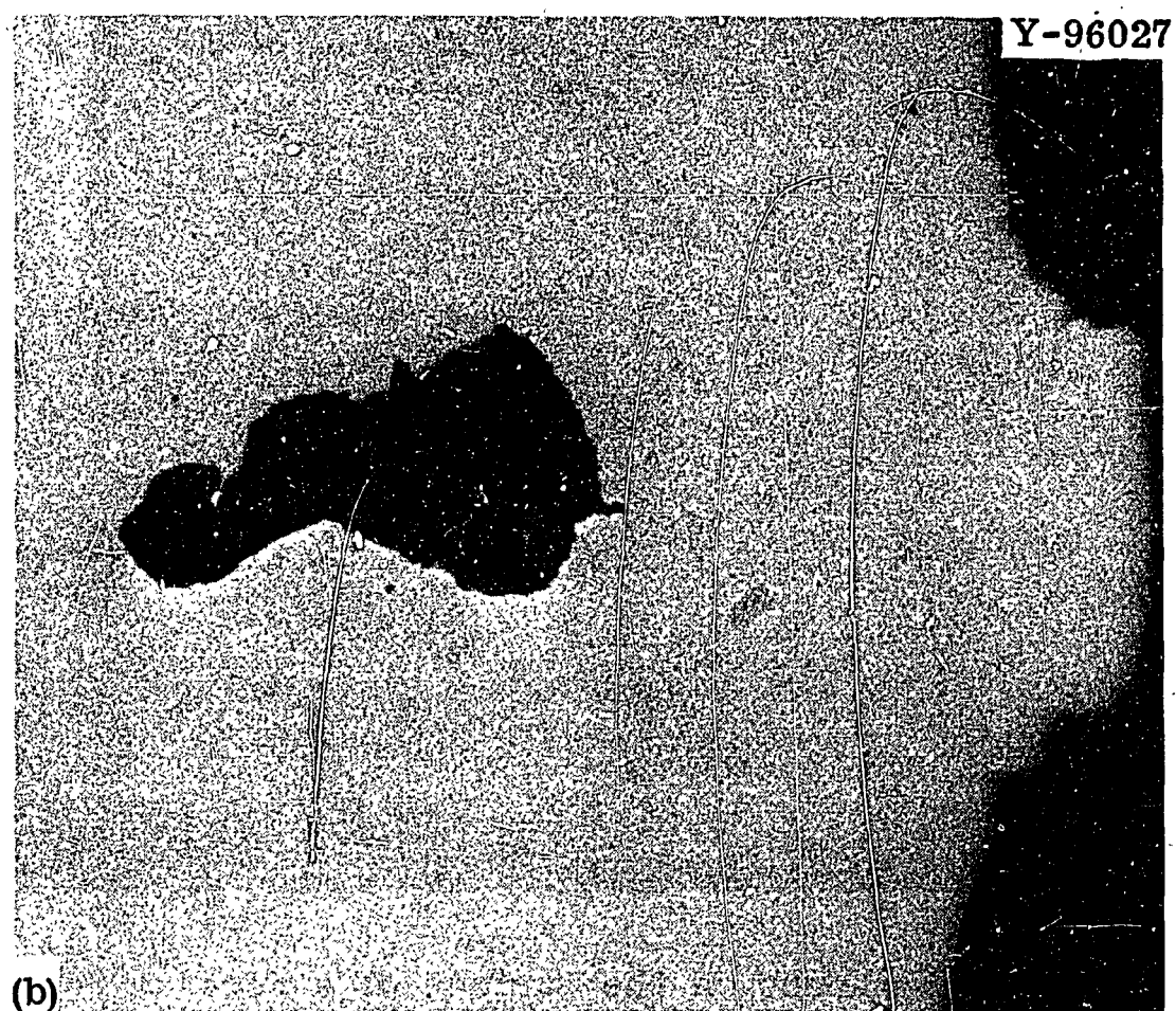
Fig. 11. Cross Section of Specimen Shown in Fig. 10 Showing How the Protuberences Were Formed. Unetched. (a) 100X. (b) 500X. [Ref: A. P. Litman, The Effect of Oxygen on the Corrosion of Niobium by Liquid Potassium , ORNL-3751 (July 1965).]
