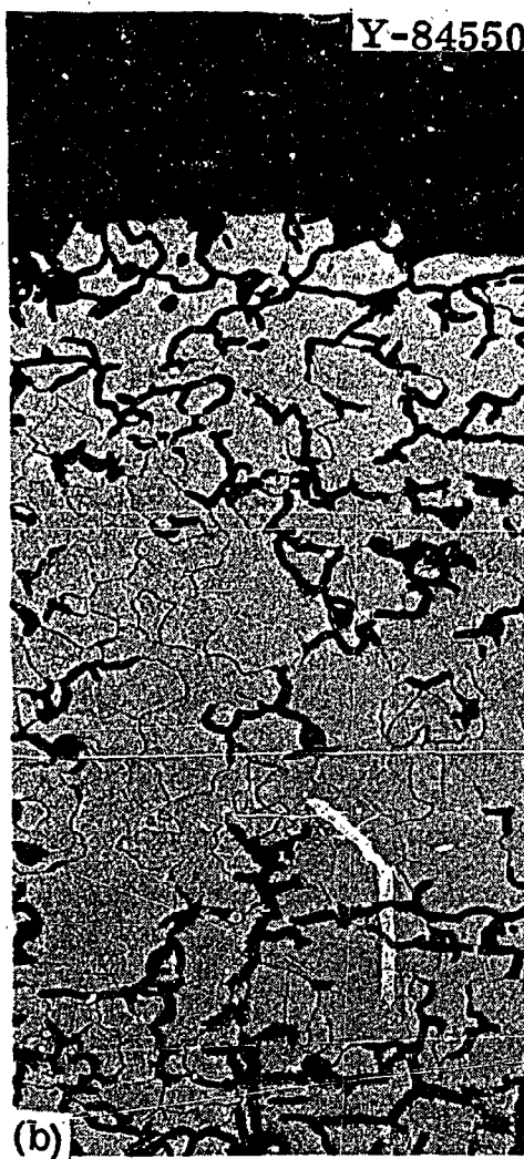
Fig. 3. Tantalum Specimens Exposed to Alkali Metals for 500 hr at 600°C. 100X. Etchant: \text{H}_2\text{O}-\text{HNO}_3-\text{NH}_4\text{HF} . (a) Initially 1300 ppm O; exposed to potassium. (b) Initially 1400 ppm O; exposed to sodium. (c) Initially 1200 ppm O; exposed to lithium.
