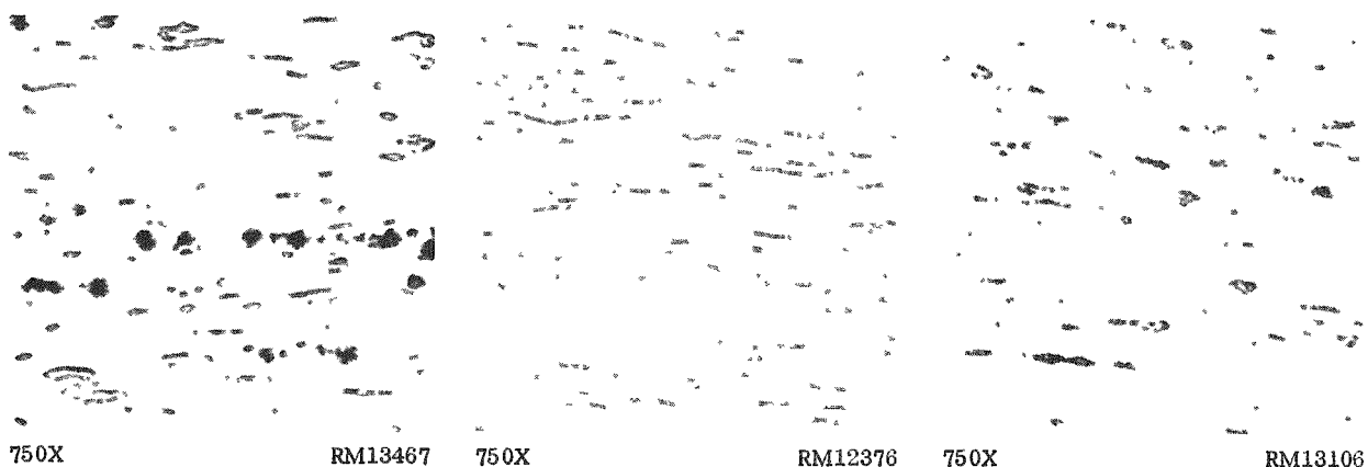
d. 10 w/o Uranium Induction Cast and Cold Reduced 80 Per Cent
