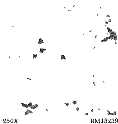
h. 10 w/o Uranium Induction Cast, Heated 1 Hr at 1000 C, and Water Quenched
