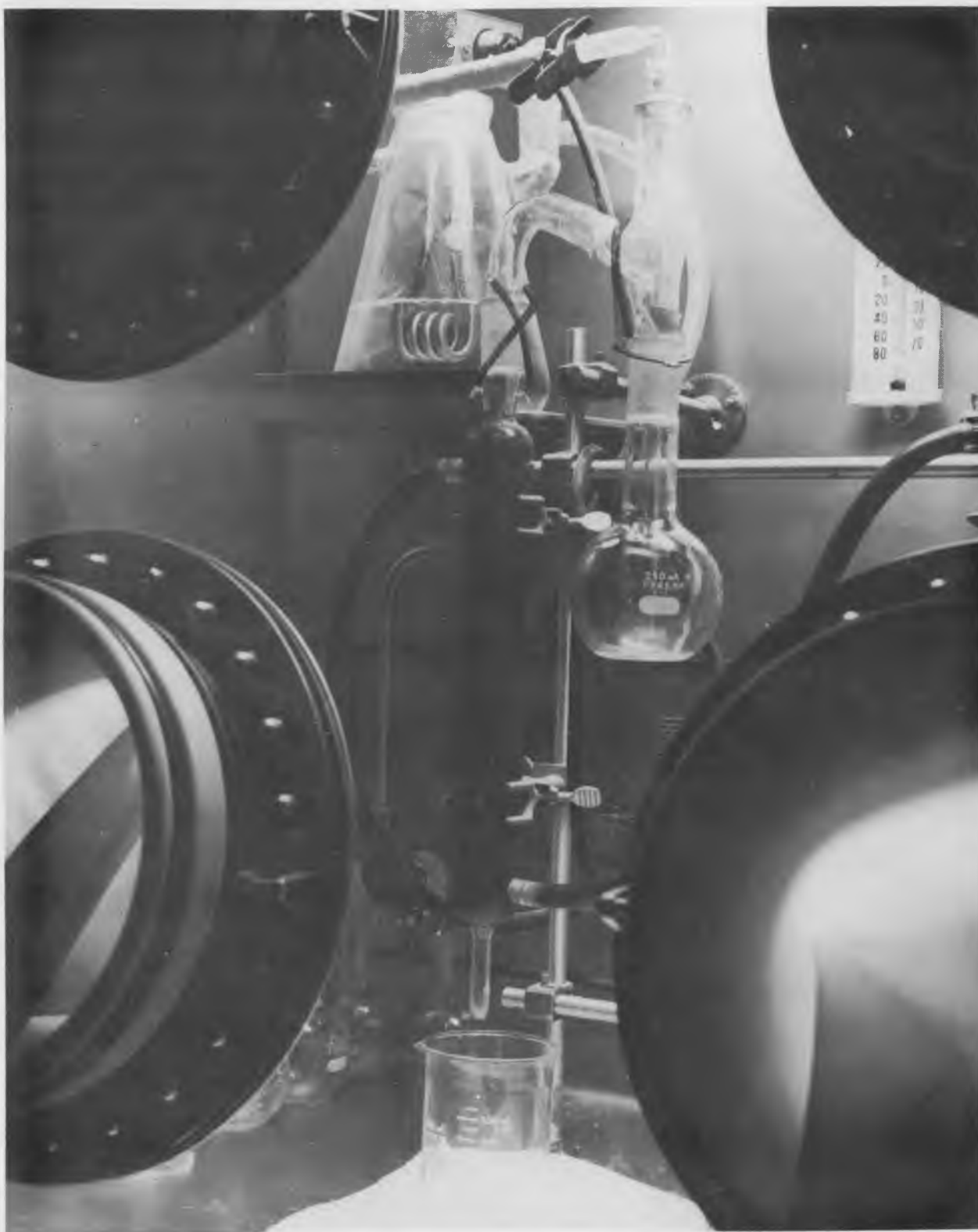
Figure 6. Distillation Apparatus for Determination of Nitrogen in \text{ThO}_2 and ^{233}\text{UO}_2 - \text{ThO}_2 (Operational Chemistry Laboratory)
