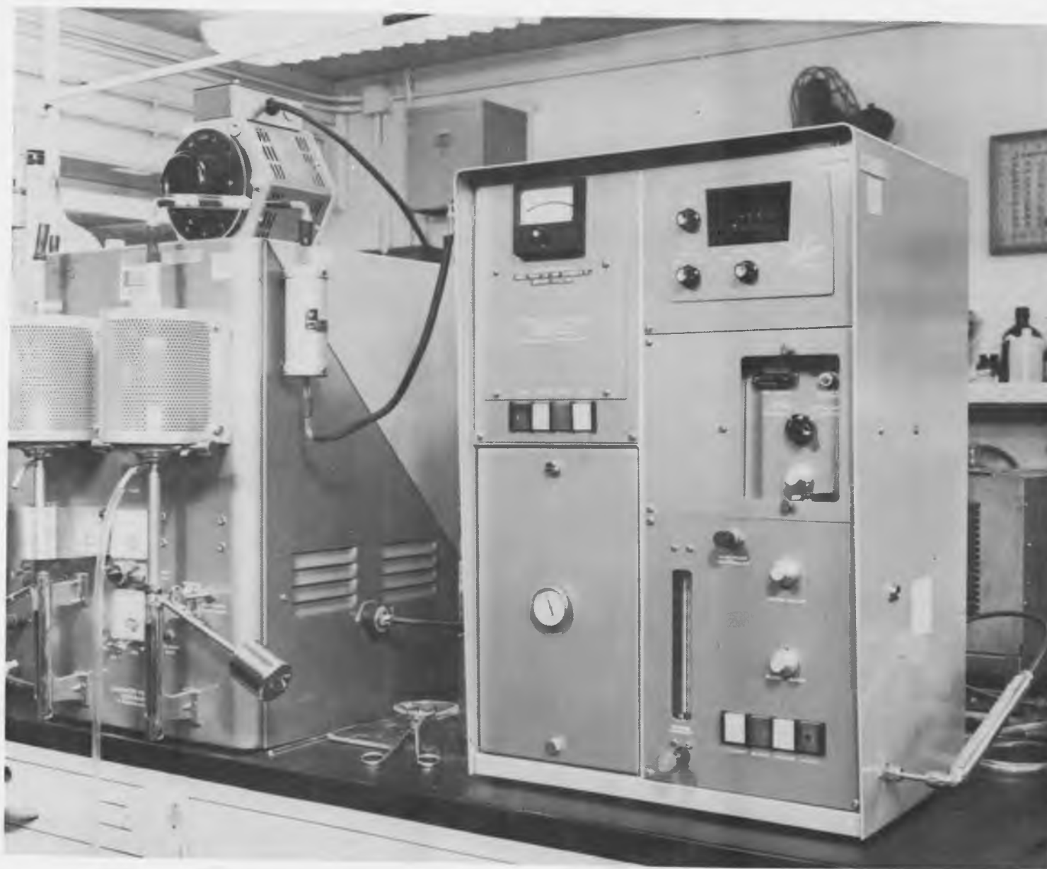
Figure 3. Instrumentation for Determination of Carbon in ThO 2 (Analytical and Spectrochemical Analysis Laboratory)
