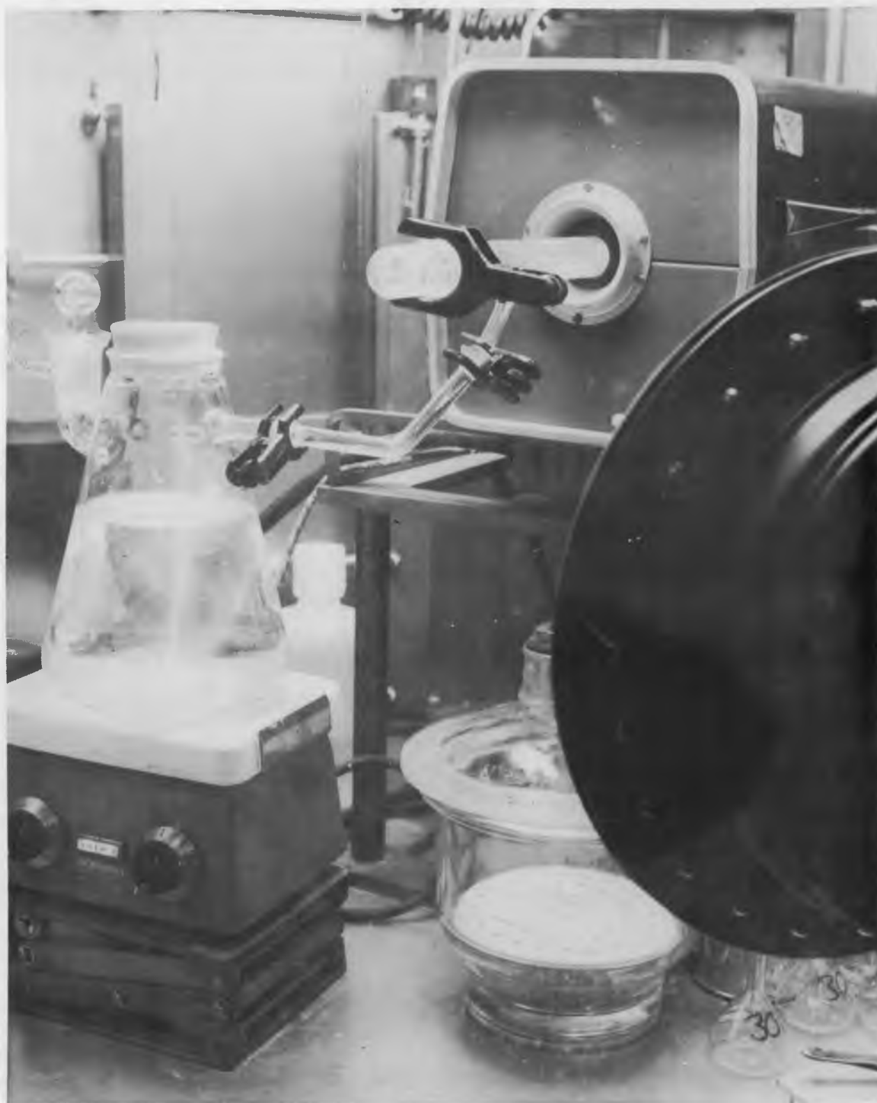
Figure 8. Pyrohydrolysis Unit for Steam Distillation of Chloride and Fluoride from ThO 2 and 233 UO 2 -ThO 2 (Operational Chemistry Laboratory)
