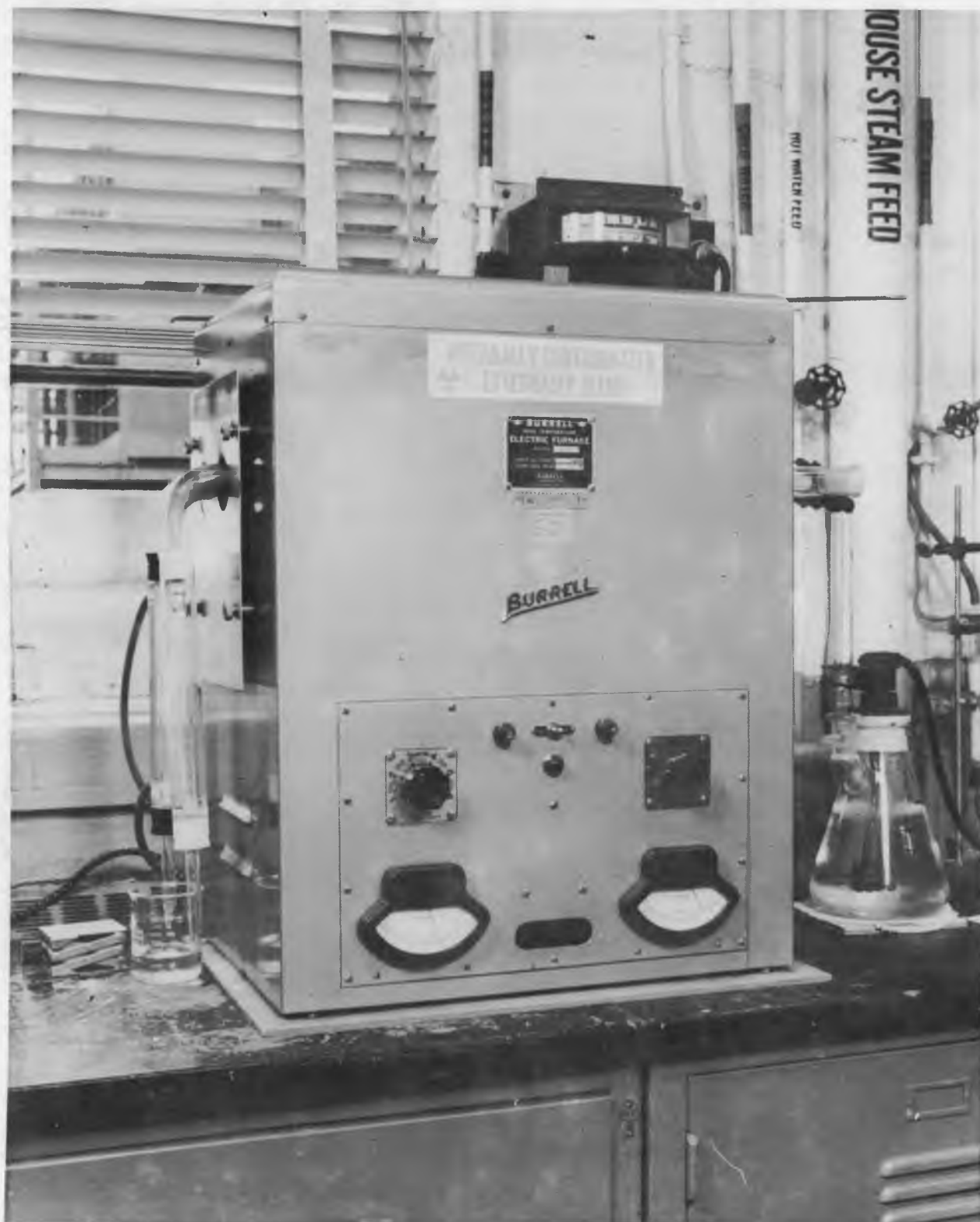
Figure 7. Pyrohydrolysis Unit for Steam Distillation of Chloride and Fluoride from \text{ThO}_2 (Analytical and Spectrochemical Analysis Laboratory)
