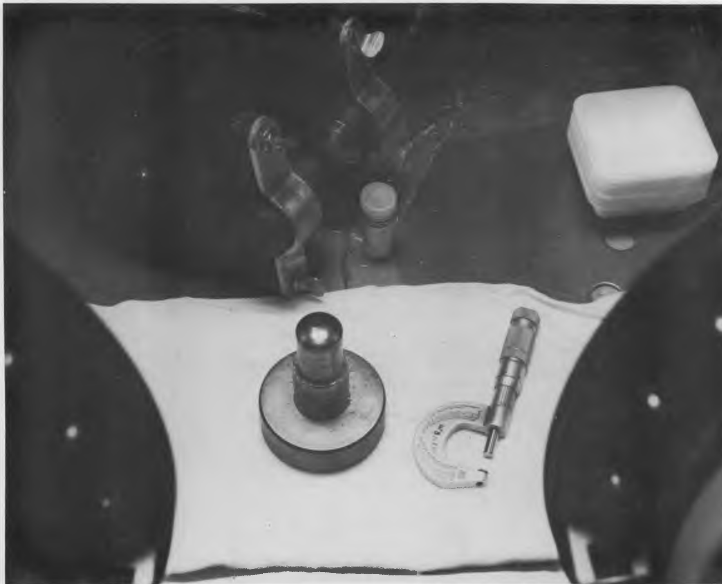
Figure 10. Plattner Mortar and Pestle and Adjustable Gap Magnet Used for Total Uranium Sample Preparation
