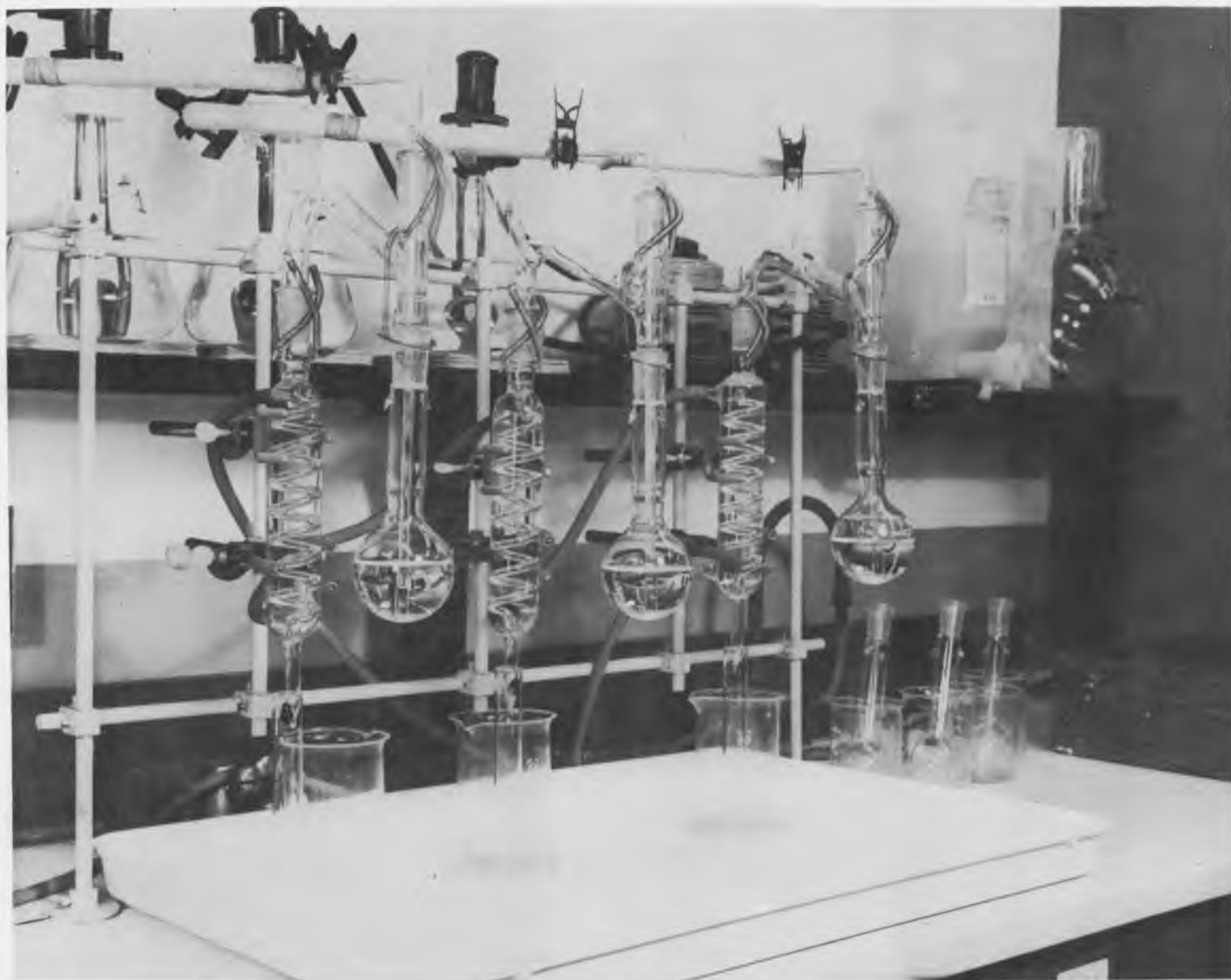
Figure 5. Distillation Apparatus for Determination of Nitrogen in \text{ThO}_2 (Analytical and Spectrochemical Analysis Laboratory)
