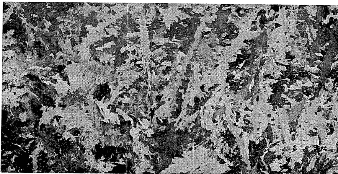
FIGURE 15-9 CAST STRUCTURE AFTER ALPHA ANNEALING AT 640°C SLUG NO. 12. BRIGHT FIELD: CONC HCl ETCH, CONC HNO 3 RINSE (3X)
