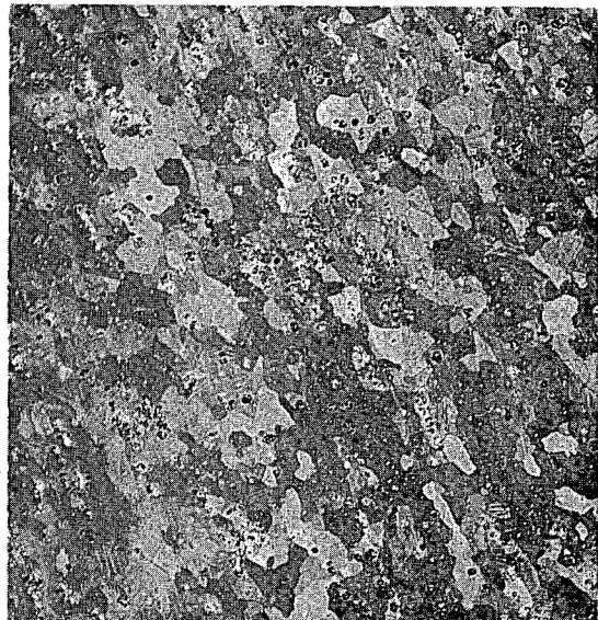
FIGURE 12-2 GRAIN STRUCTURE OF SLAB F-8142. (100X, POLARIZED) TOP LEFT: BACK END OF SLAB AT CENTER; LONGITUDINAL SECTION TOP RIGHT: BACK END OF SLAB AT EDGE; LONGITUDINAL SECTION BOTTOM LEFT: LEAD END OF SLAB AT CENTER; LONGITUDINAL SECTION BOTTOM RIGHT: LEAD END OF SLAB AT EDGE; LONGITUDINAL SECTION
