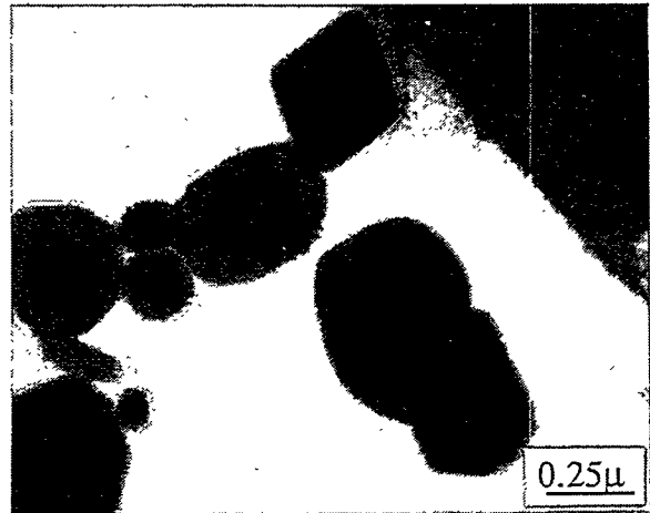
Figure 6. TEM microstructure in the simulated HAZ with a peak temperature of 900°C.
