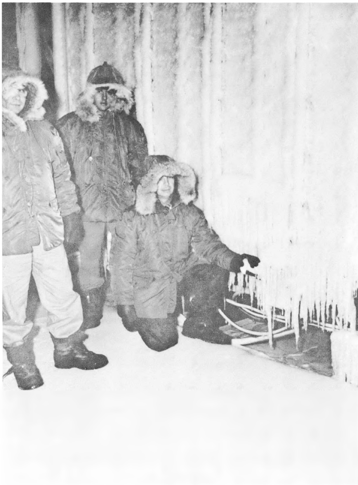
Fig. I-12. Heavily Iced Condenser Test Model and Test Personnel at -45^{\circ}\text{F}
