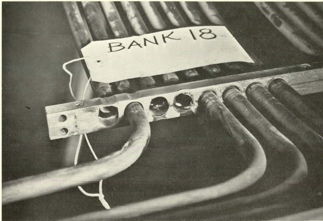
Fig. 11. EFAPP Steam Generator: Enlargement of Support-bar Holes due to Tube-to-Support-bar Impacts. (From Ref. 26.)
