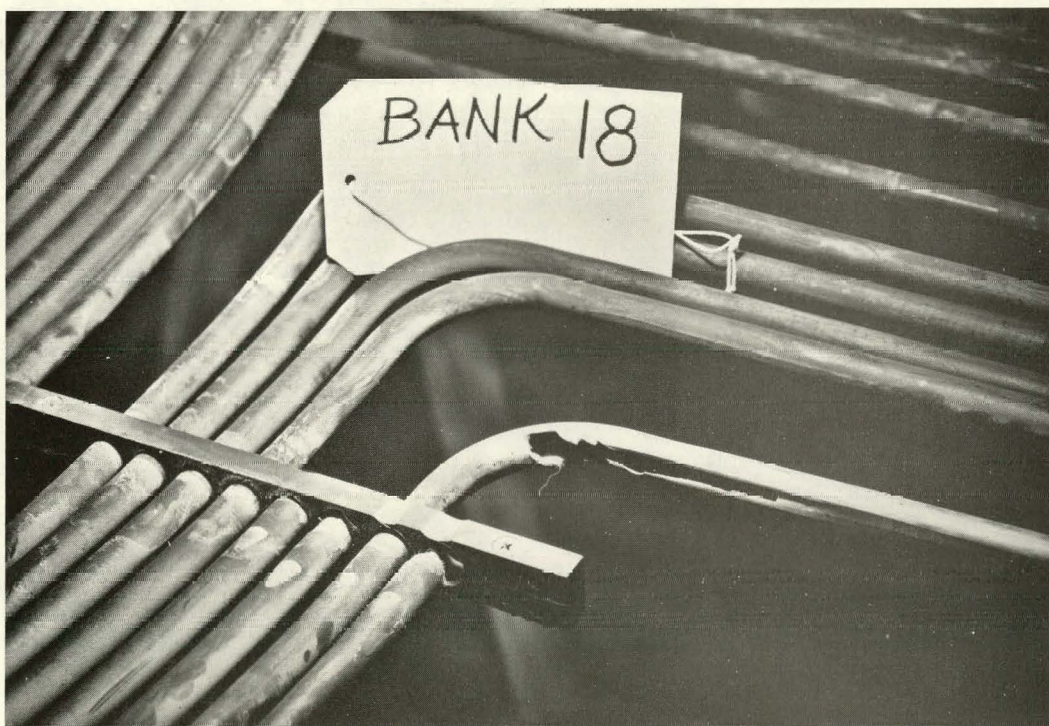
Fig. 10. EFAPP Steam Generator: Tube Crack due to Collision with Adjacent Tubes. (From Ref. 26.)
