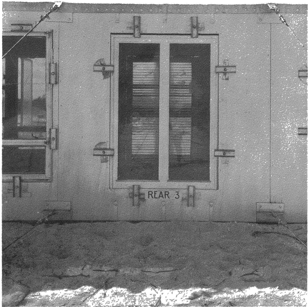
FIG. 3.45 Outside of Casement Window 13 before the Blast. This is a duplicate of window 5 except that the left-hand sash was glazed with tempered glass and the right-hand sash with wire glass.
