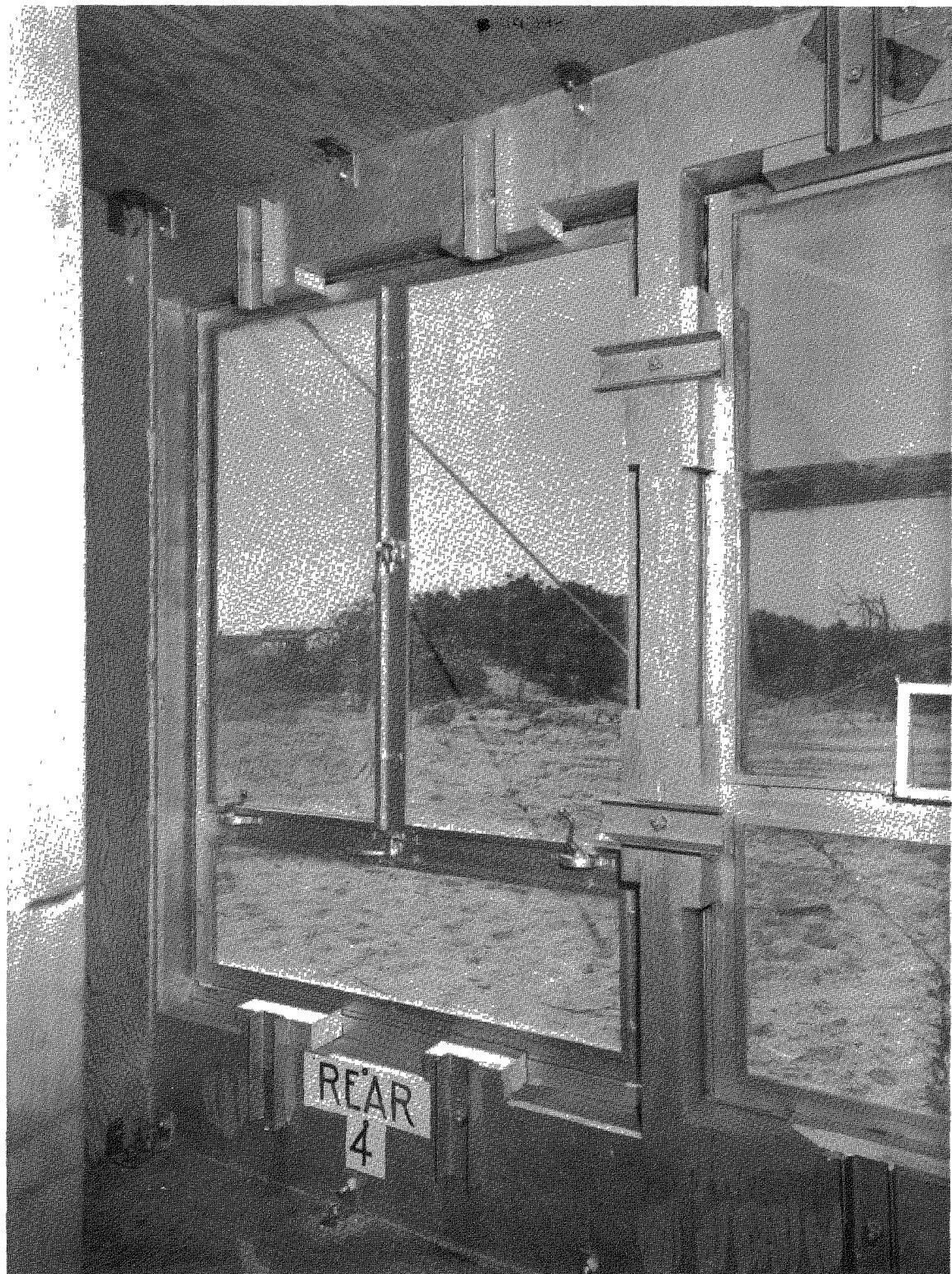
FIG. 3.51 Inside of Casement Window 14 before the Blast
