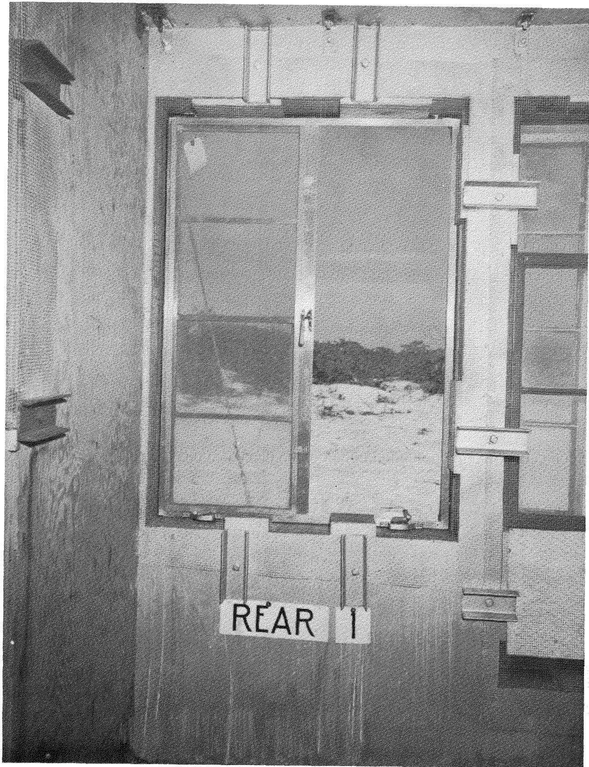
FIG. 3.40 Inside of Casement Window 10 after the Blast
