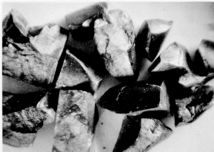
FIGURE 9. UN IRRADIATED AT A MAXIMUM CENTER-LINE TEMPERATURE OF 650 C TO AN URANIUM BURNUP OF 2.1 a/o (SPECIMEN 11A FROM CAPSULE BMI-40-5)
