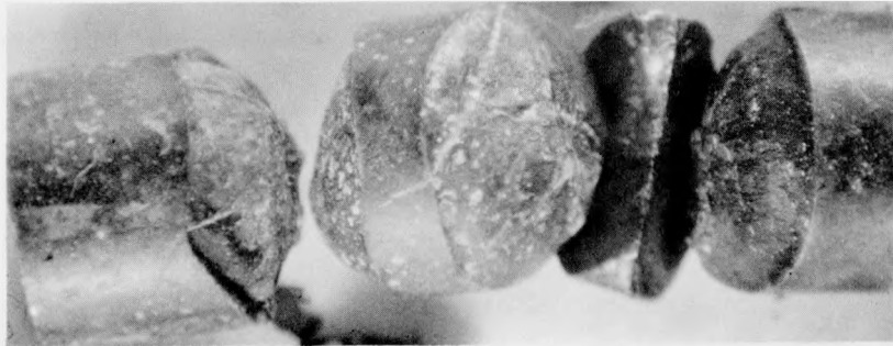
FIGURE 8. UN IRRADIATED AT A MAXIMUM CENTER-LINE TEMPERATURE OF 200 C TO AN URANIUM BURNUP OF 0.34 a/o (SPECIMEN 19 FROM CAPSULE BMI-40-4)
