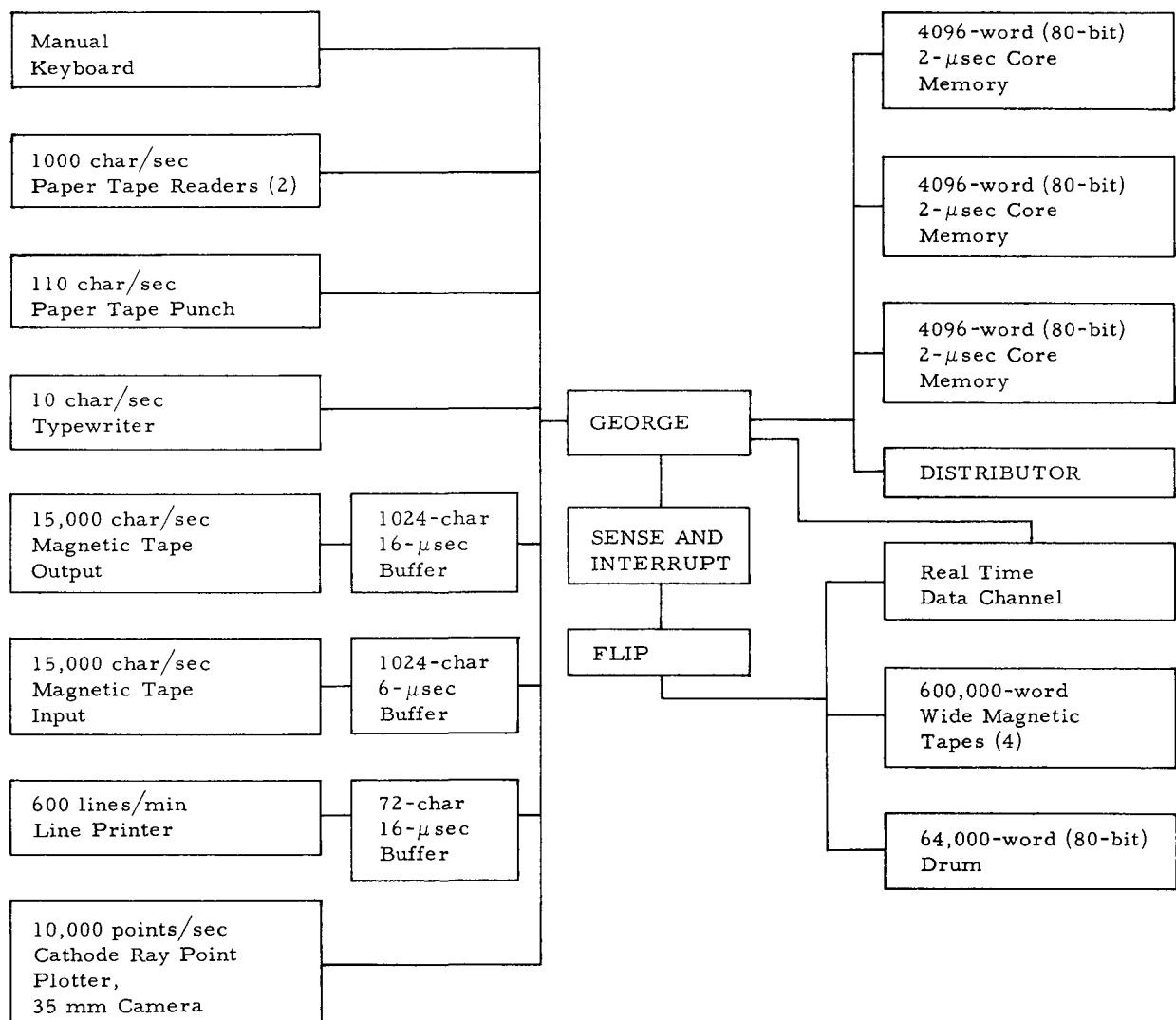
An automatic data-processing system, known as CHLOE, for analyzing spark-chamber photographs has been developed. It utilizes a fiber optics cathode-ray-tube scanner and an ASI-210 digital computer.
