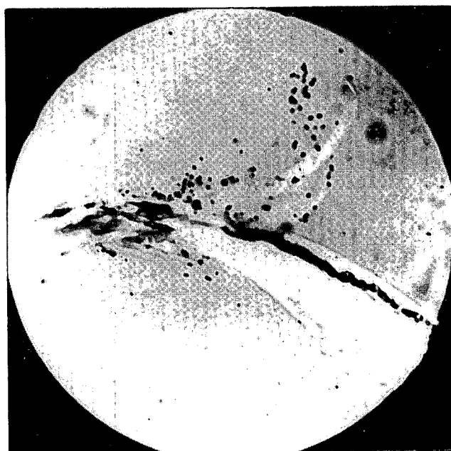
FIGURE 21 AUTORADIOGRAM IN LIQUID EMULSION OF A PORTION OF A SINGLE FIBER CONTAINED IN A MICROTOME SECTION OF SAMPLE No. 732
