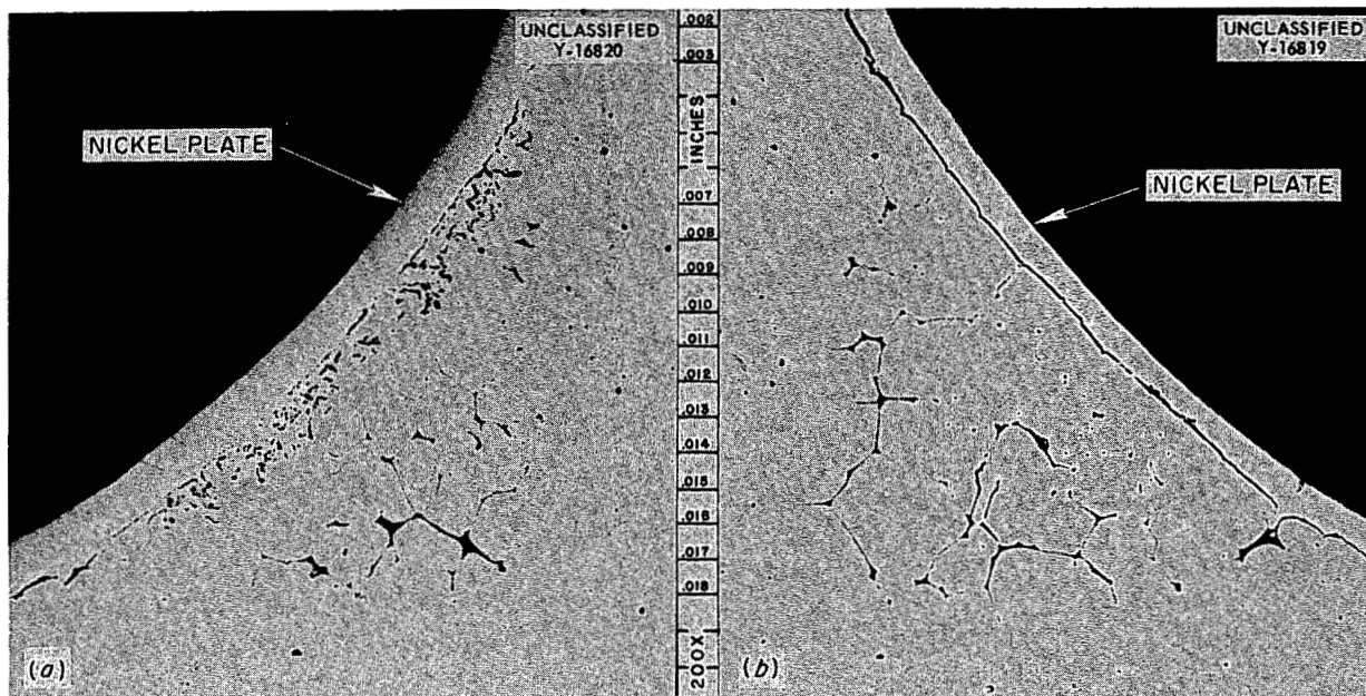
Fig. 7. Brazing Alloy 75% Ni-25% Ge After Seesaw Test at 1500°F for 100 hr in (a) Sodium and (b) \text{NaF-ZrF}_4\text{-UF}_4 (50-46-4 mole %). The 2-mil attack which occurred in both media is shown. Both specimens were nickel-plated after the test in order to preserve edges during polishing. Etchant: citric acid. 200X. Reduced 16%. (Secret with caption)
