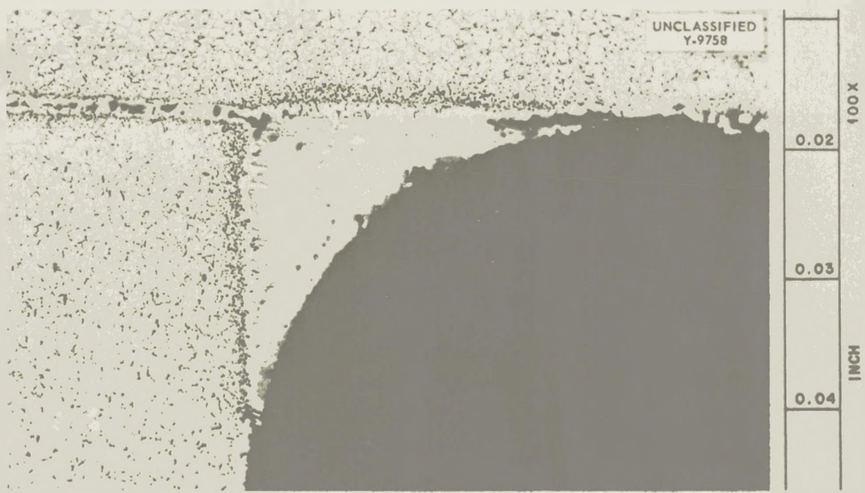
Fig. 7.4. "Electroless" Ni-P Brazed Type 316 Stainless Steel T Joint, Tested in Air for 500 hr at 800°C. 100X.
