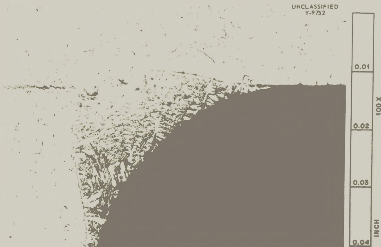
Fig. 7.7. Chromium-Coated "Electroless" Ni-P Brazed Type 316 Stainless Steel Joint Tested in Sodium for 100 hr at 816°C. 100X.
