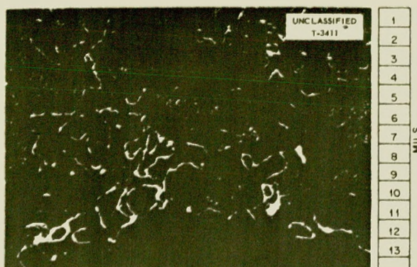
Fig. 6.5. Deposit on Graphite Rod After 500 hr in an Inconel Loop Circulating NaF-ZrF_4-UF_4 (50-46-4 mole %) at 1500^\circ F . 250X. Reduced 39%.
