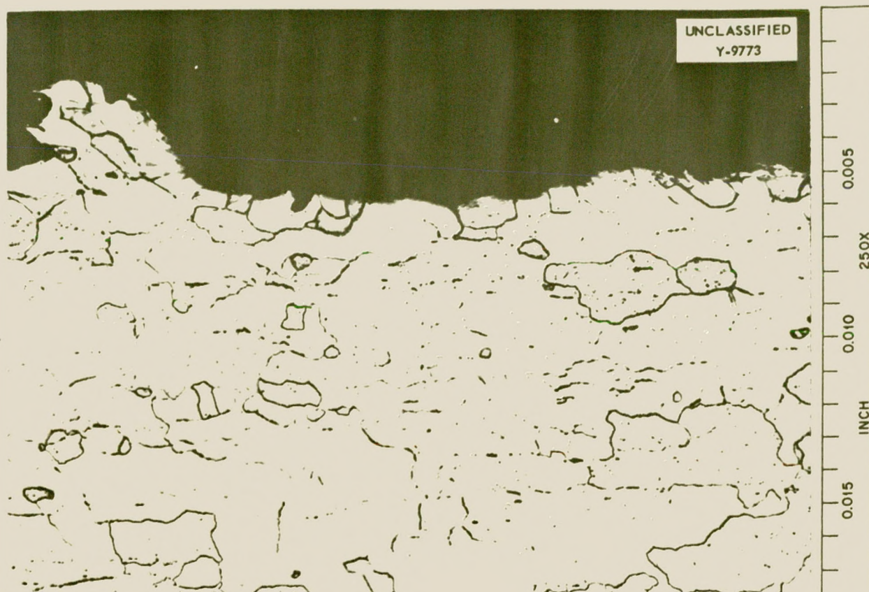
Fig. 6.7. Hot Leg of Type 410 Stainless Steel Loop After Circulating Lead for 545 hr at 810°C. 250X.
