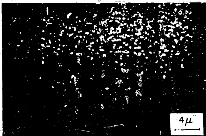
Fig. 17 SEM micrograph showing the precipitates in the banded structure of Inconel 718 (Heat 83C2EK) heat treated to condition B. Precipitates at the top of the micrograph represent those in the light colored bands of Fig. 16. Precipitates were not distinctly resolved in the dark bands. Etchant No. 1 4200X
