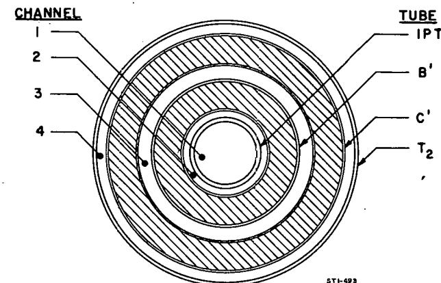
Figure 1. Cross Sections of UO<sub>2</sub> Tube Assemblies for Physics Tests
