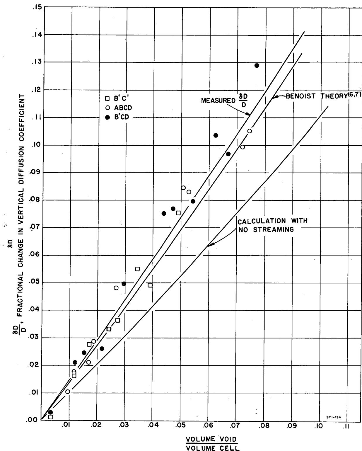
Figure 2. Change in Vertical Diffusion Coefficient on Voiding Coolant Channels in  $\text{UO}_2$  Tube Clusters
