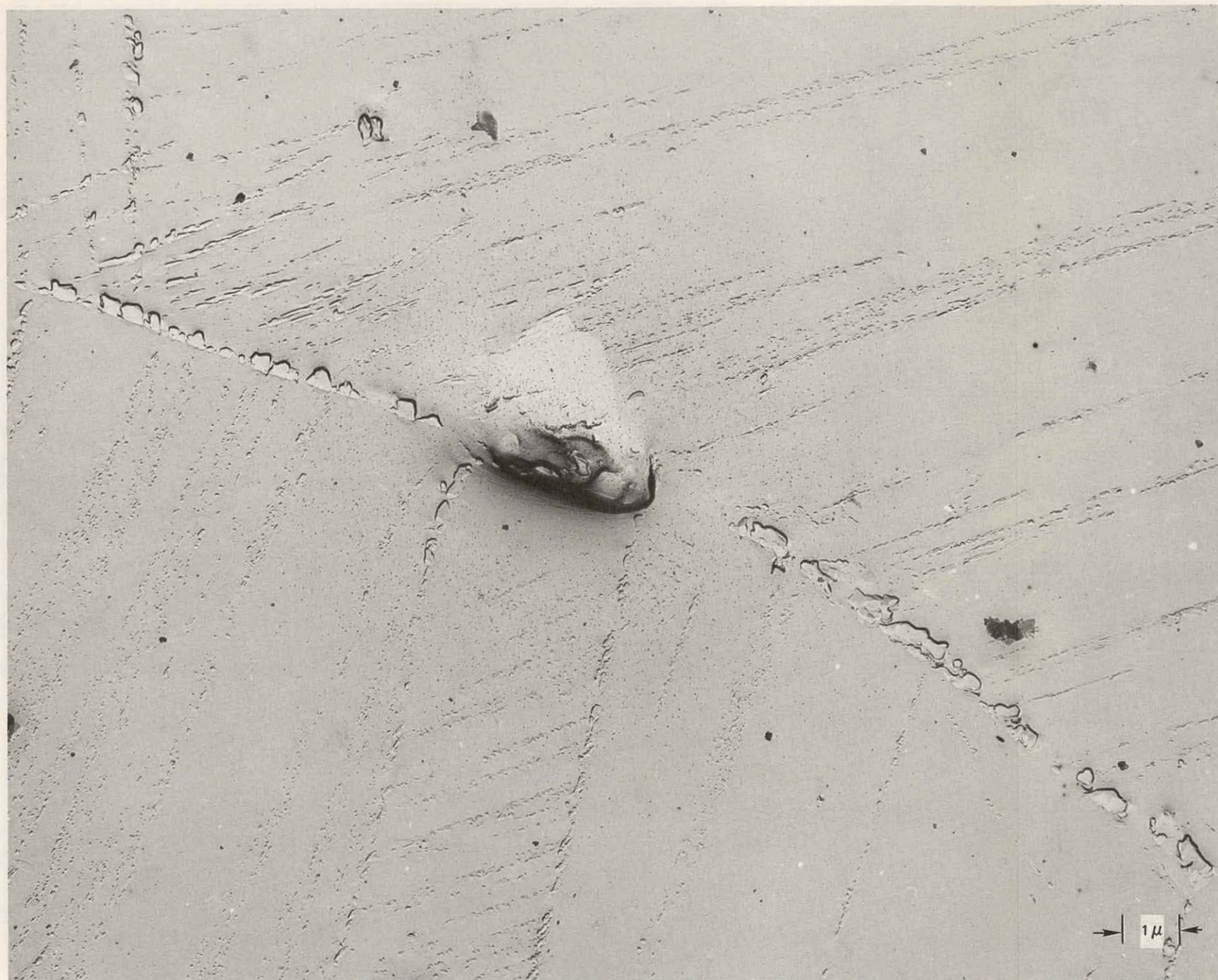
a. No Helium, Rupture Life = 683 hr, Elongation = 5%
