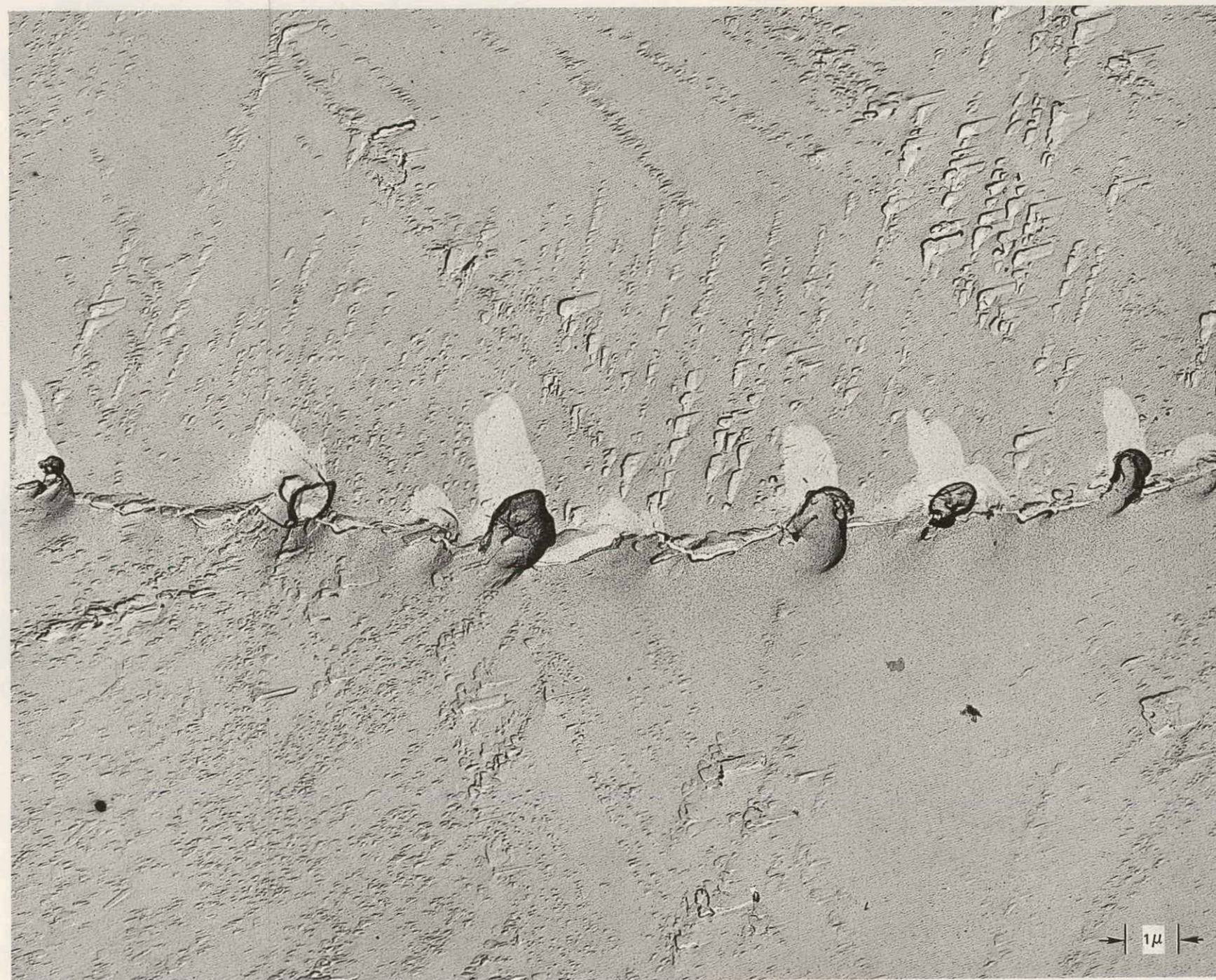
b. 4.0 \times 10^{-5} atom fraction Helium, Rupture Life = 173 hr, Elongation = 2%
