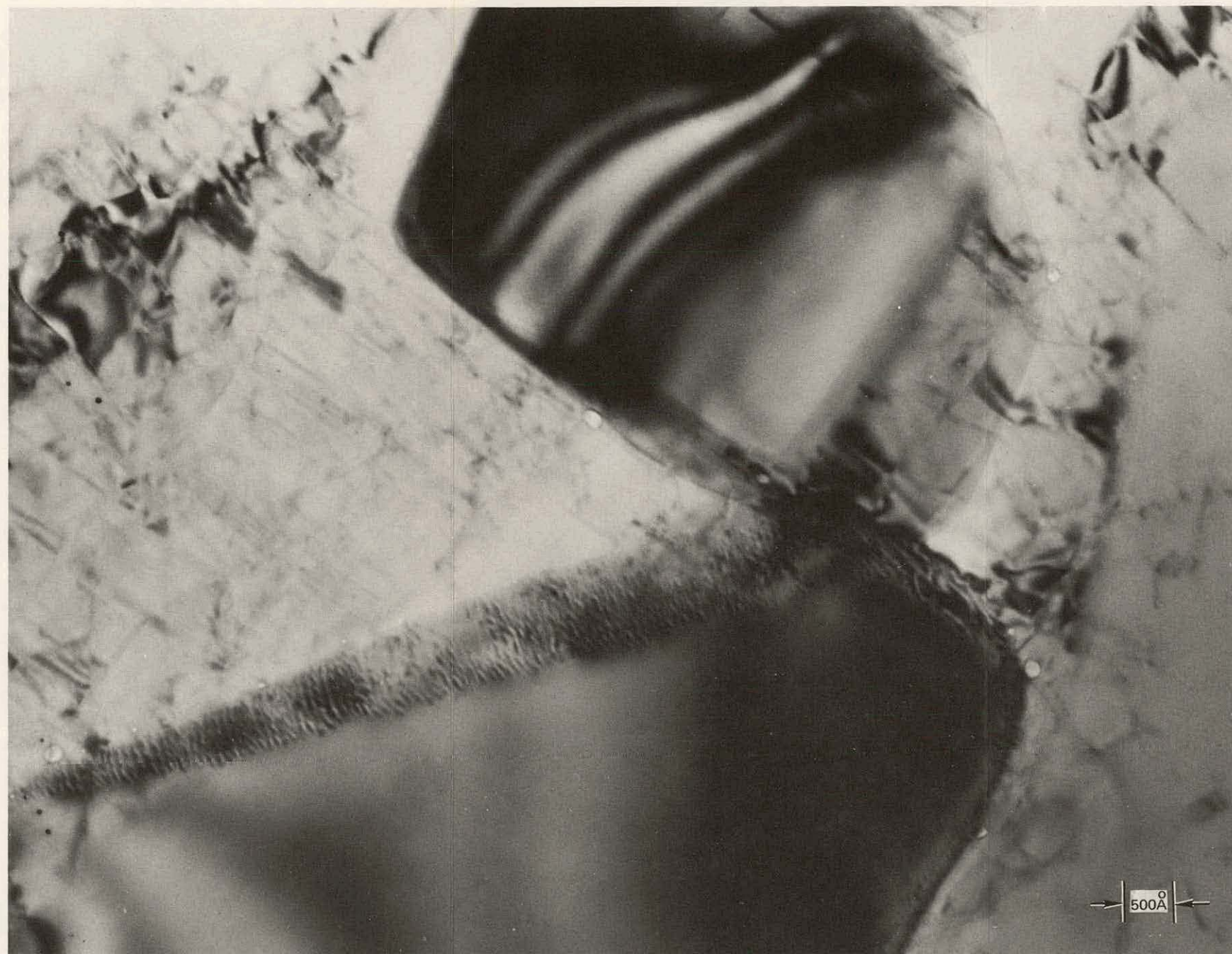
a. 1.5 \times 10^{-6} atom fraction Helium, Rupture Life = 419 hr, Elongation = 17%
