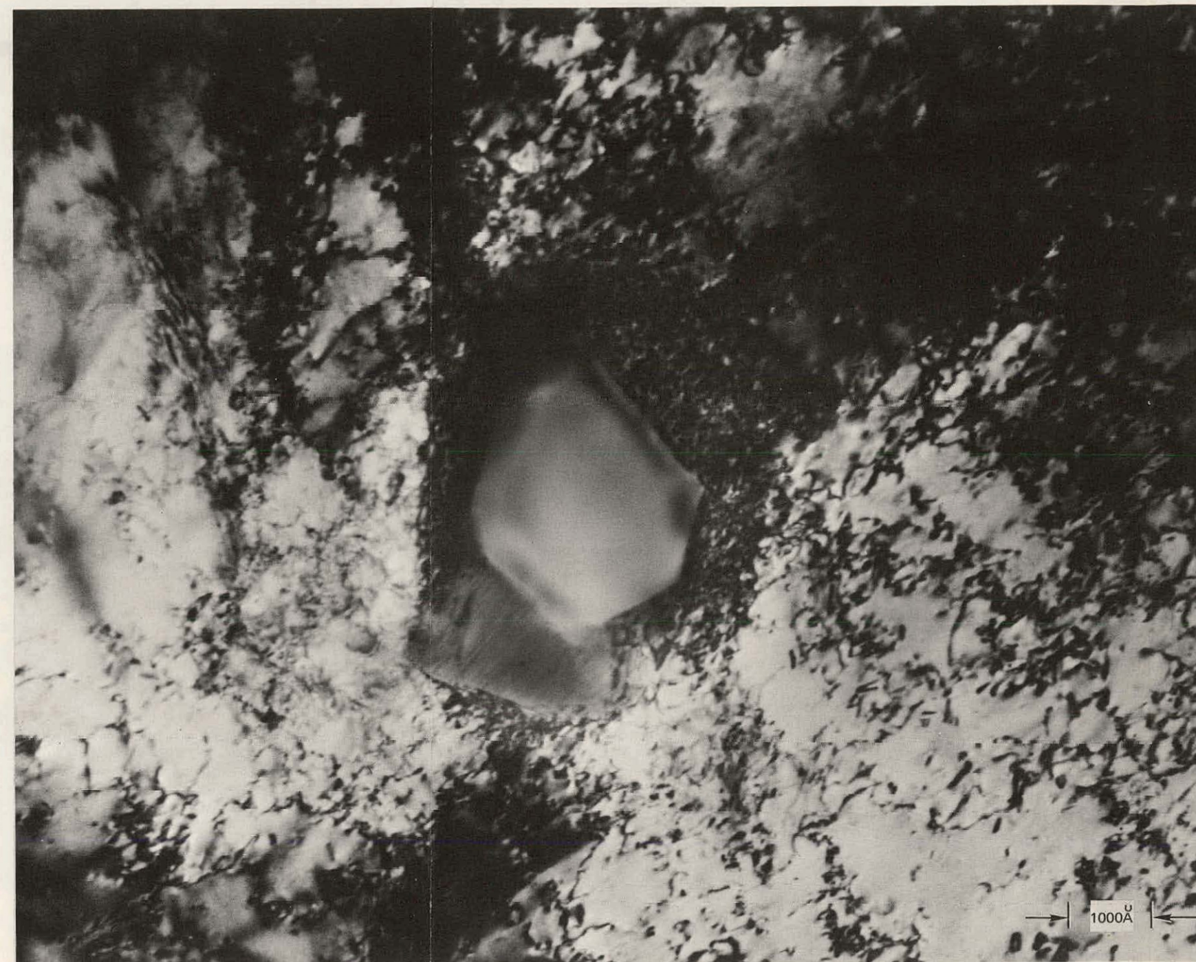
Figure 10. Type 316 Stainless Steel (Treatment 6) Containing 4.0 \times 10^{-5} atom fraction Helium, Tested at 700°C, Showing Growth of Sigma Phase on M_{23}C_6 Particle. Rupture Life = 594 hr, Elongation = 10%
