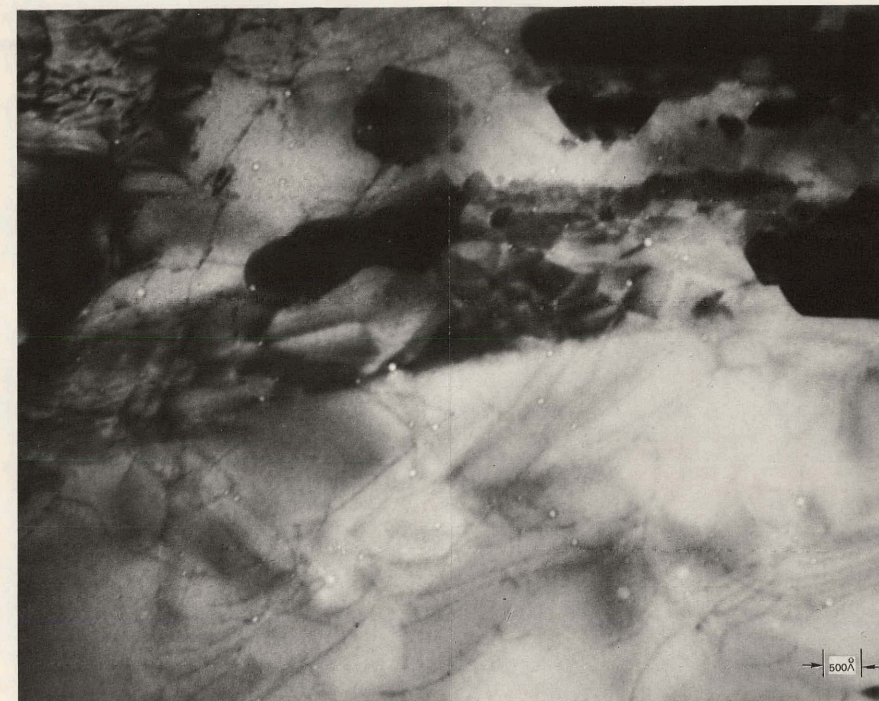
Figure 11. Type 316 Stainless Steel (Treatment 13) Containing 4.0 \times 10^{-5} atom fraction Helium, Tested at 700°C, Showing Helium Bubbles in Matrix and in Prior Slip and Deformation Bands. Rupture Life = 173 hr, Elongation = 2%
