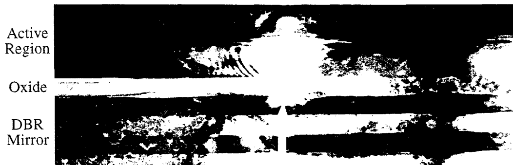
Fig. 3. Cross section TEM image of \text{AlAs} oxide aperture where arrow denotes the oxide terminus.
