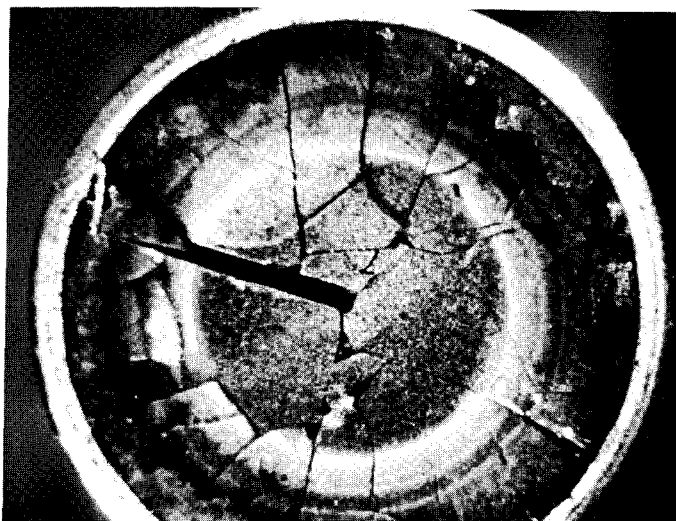
FIGURE 17: Longitudinal Slit, Showing Essentially No Change in Shape Except Rounding at Tip. Element CEZ. Reference 6551
