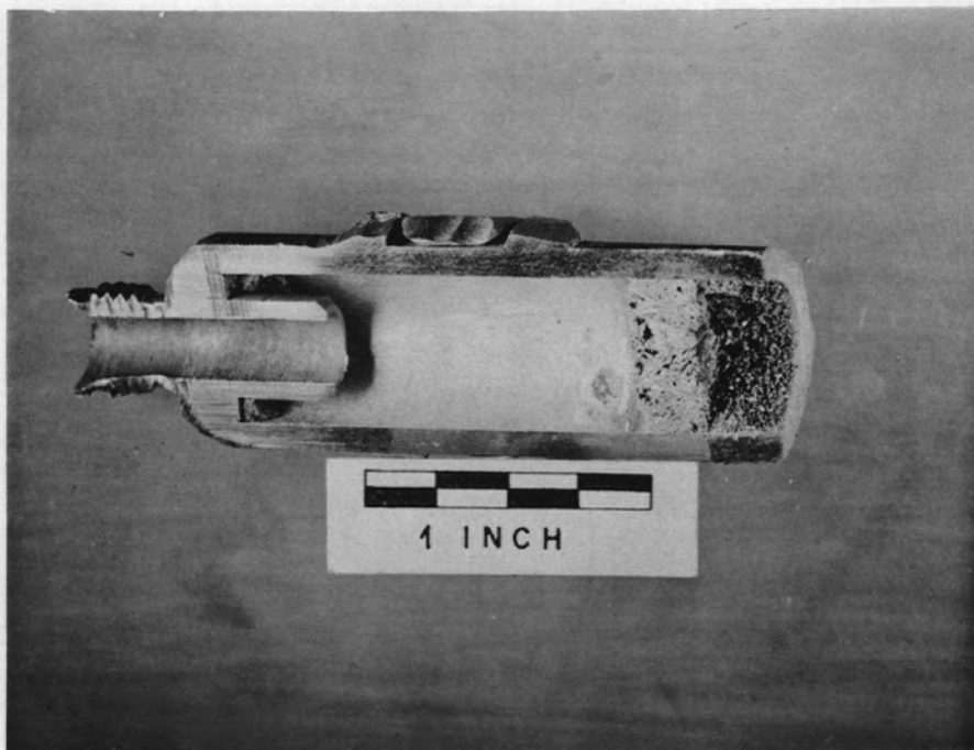
Fig. 86 (T-5211) Layer of Chromium Crystals Found in the Trap of an Inconel Loop after Circulating Fused Fluorides for 5000 Hr at 1500°F. Unclassified - Secret with caption.
