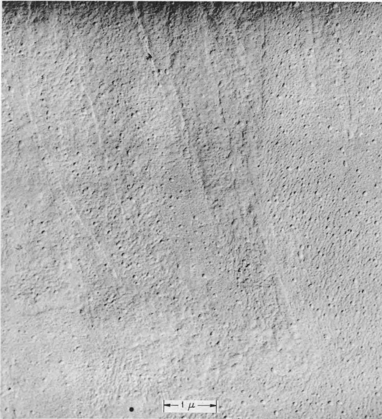
Fig. 15. Surface of Zirconium Test Specimen Opposite to Side Seeing Fission Fragment Recoils (Exposed in Neutron Flux Only; Pd Shadowed Carbon Replica).
