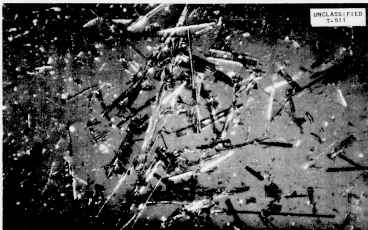
Fig. 11.17. Deposit of Silver Crystals by Mass Transfer in Silver Capsule Containing Sodium Hydroxide.
