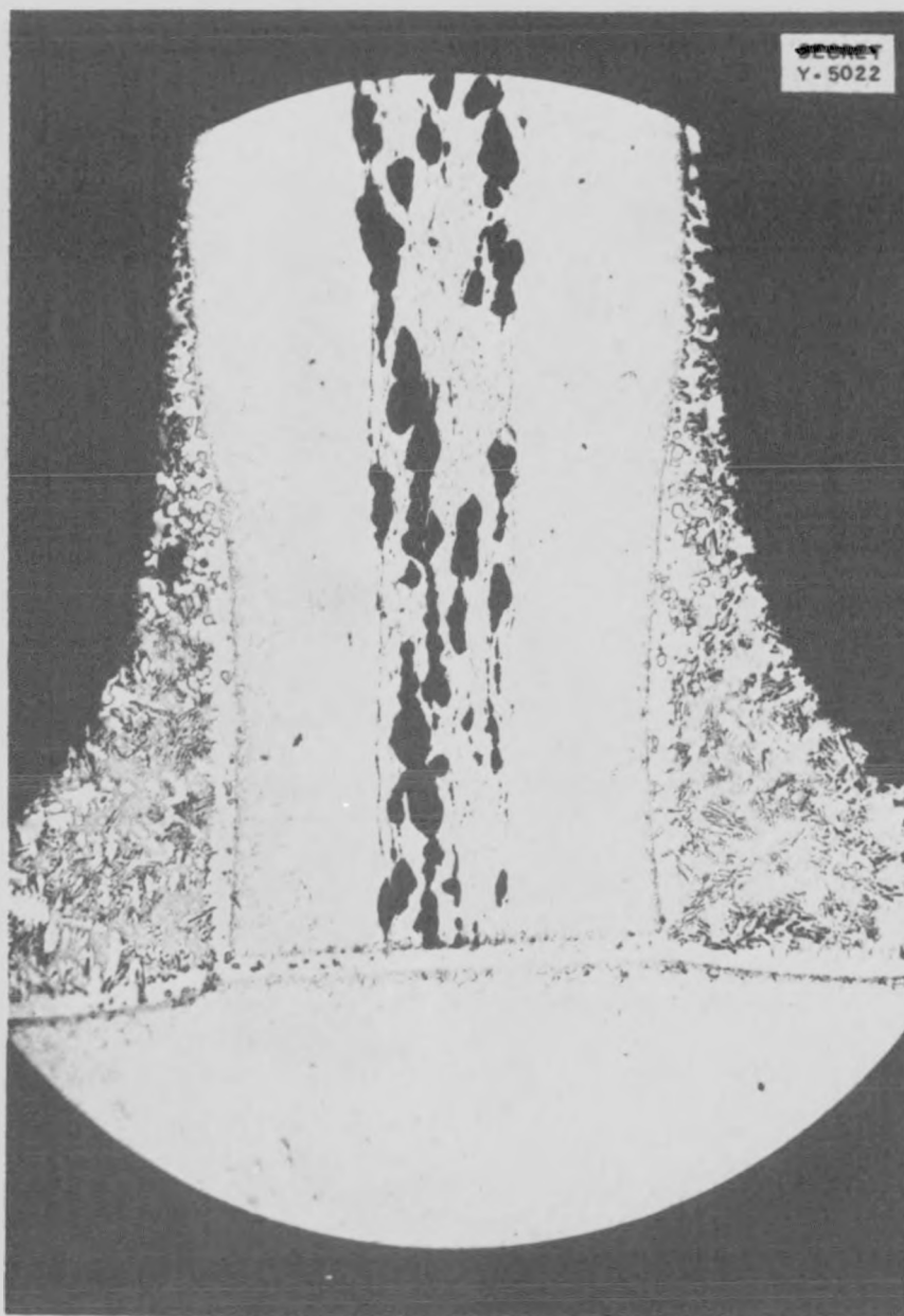
Fig. 13.8. Transverse Section of a Stainless Steel-Clad Fuel-Element Butt Microbraze to a Stainless Steel Sheet. Etchant, none. 40X.
