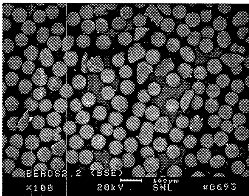
Figure 2 SEM photomicrograph of the Class V - Medium beads. A 100 \mu\text{m} reference sizing bar is included at the bottom of the photograph.
