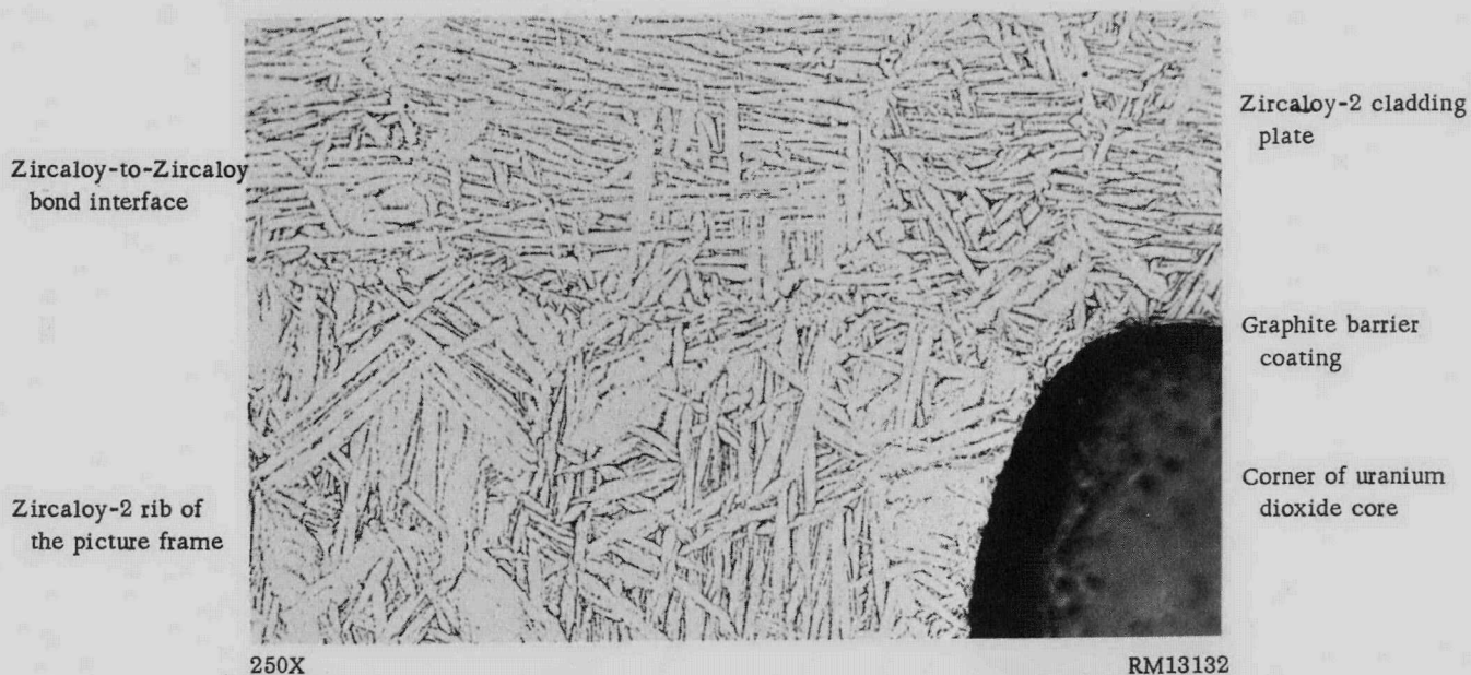
FIGURE 17. TYPICAL INTERFACE BETWEEN THE ZIRCALOY CLADDING COMPONENTS AND THE CORNER OF A URANIUM DIOXIDE CORE COATED WITH BUFFED GRAPHITE IN A PRESSURE-BONDED AND HEAT-TREATED FUEL ELEMENT
