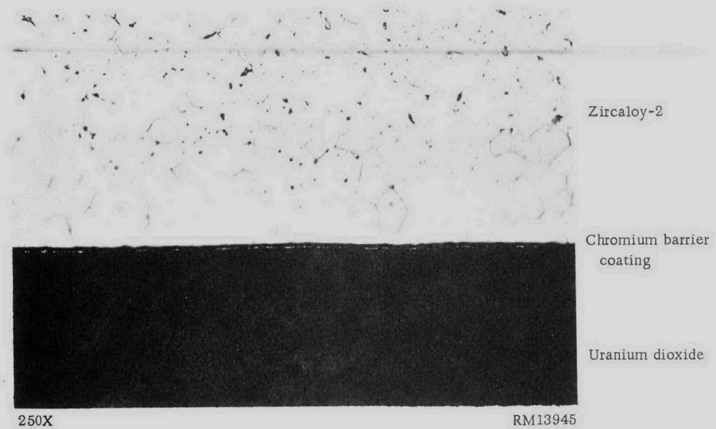
FIGURE 14. TYPICAL AS-PRESSURE-BONDED INTERFACE BETWEEN A ZIRCALOY CLADDING PLATE AND A URANIUM DIOXIDE CORE COATED WITH 25 TO 40- \mu IN. -THICK CHROMIUM BY VACUUM EVAPORATION
