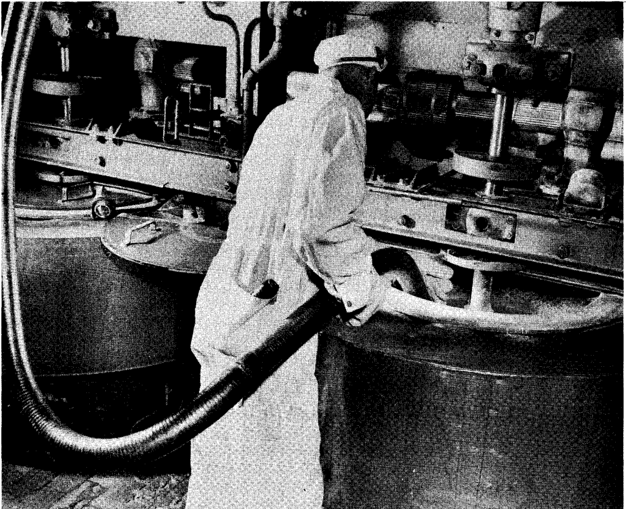
Figure II-5.3 PNEUMATIC UNLOADING, which replaced manual unloading of the denitration pots, was one of the improvements Mallinckrodt made.
