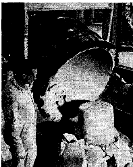
Figure II-11.4 IN THE BREAK-OUT OPERATION, the dingot, product slag and the lining were removed from the shell.
