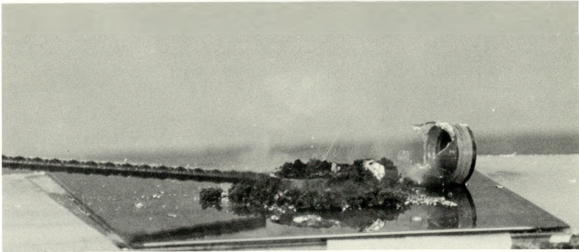
Figure 3. FIFTEEN HUNDRED GRAMS OF URANIUM POWDER IGNITING UPON EXPOSURE.
