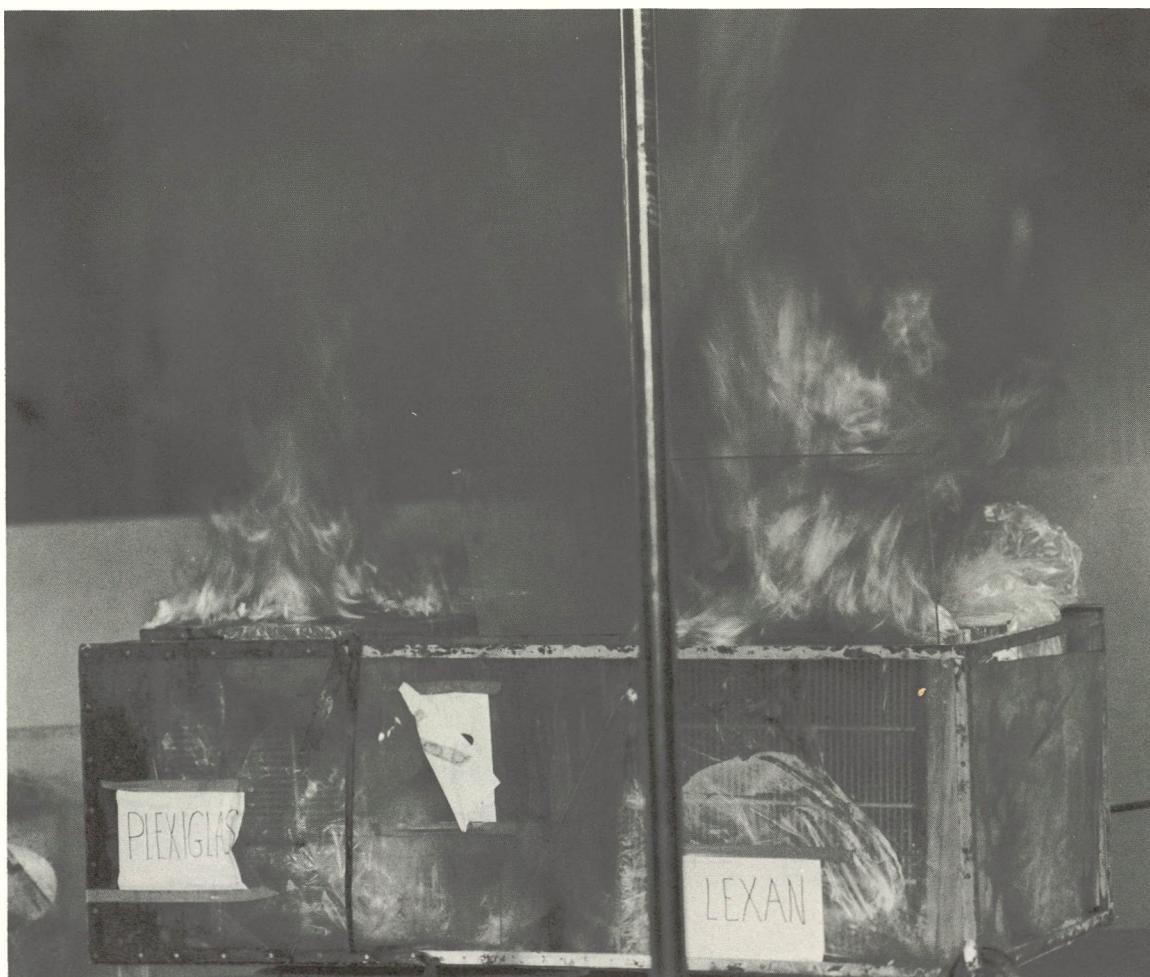
Figure 6. TESTING BURNING LITHIUM HYDRIDE POWDER UNDER SPRINKLERS.
