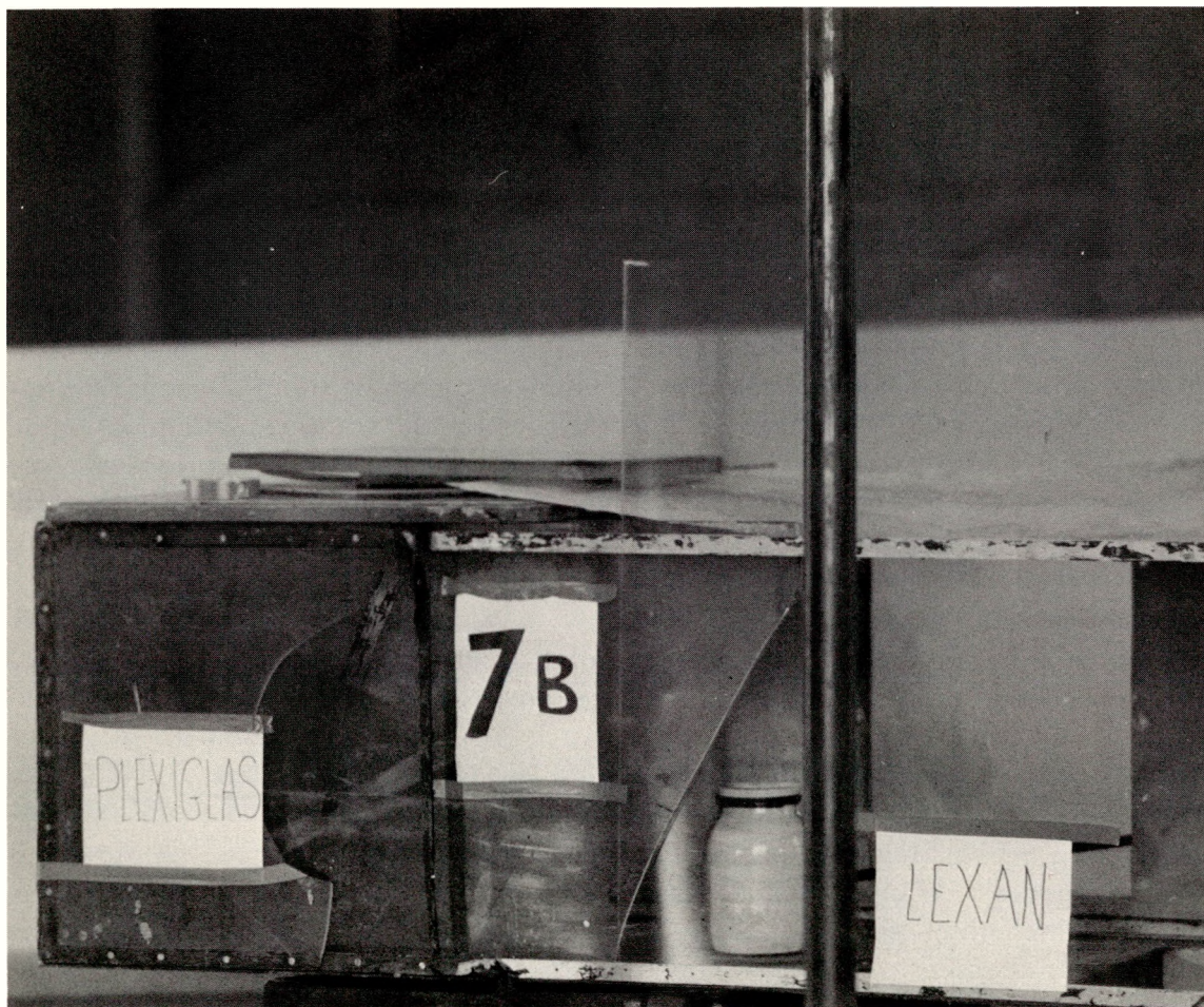
Figure 5. SIMULATED GLOVE BOX WITH A GLASS JAR CONTAINING TWO KILOGRAMS OF LITHIUM HYDRIDE POWDER.
