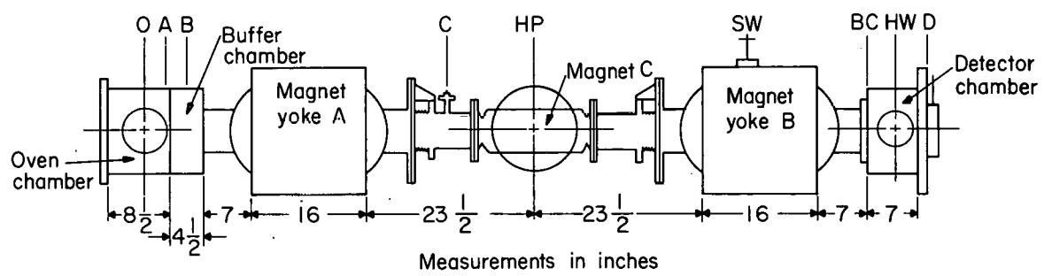
Fig. 6. Diagrammatic sketch of the physical characteristics of atomic-beam machine B.
