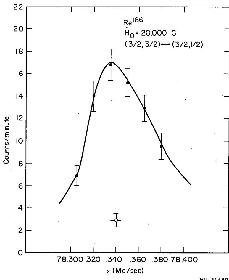
Fig. 28. Gamma transition in Re<sup>186</sup> at 20.000 G.
