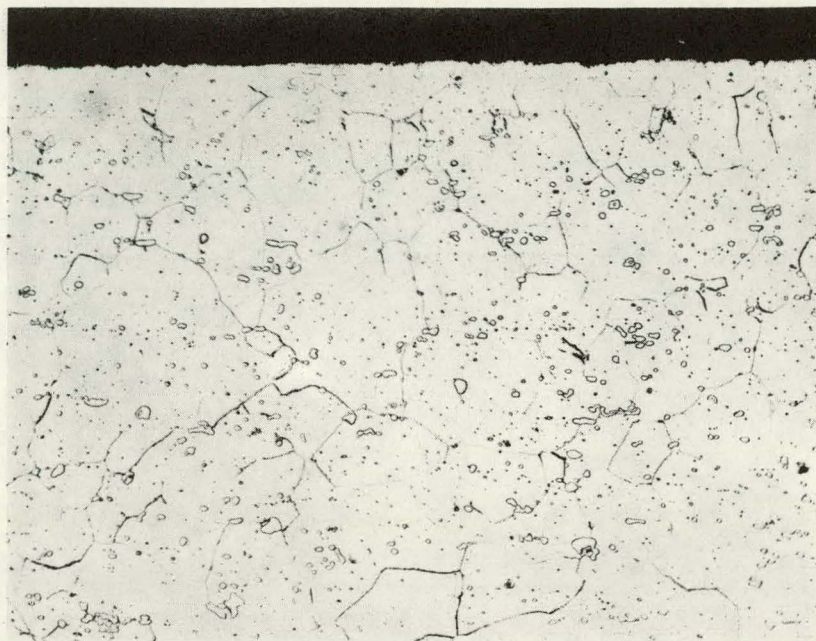
FIGURE 52 HASTELLOY X-AS-RECEIVED AT 250 X
