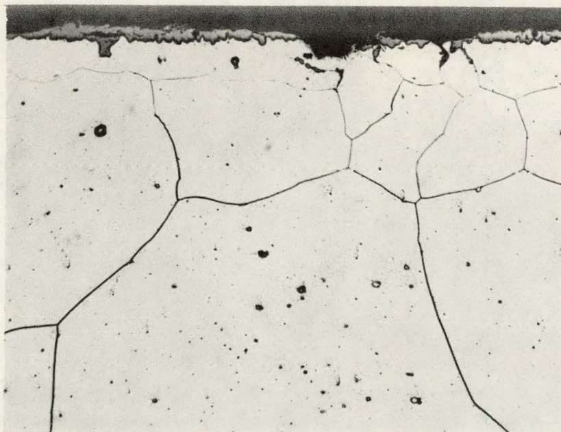
FIGURE 57 INCONEL AFTER 5000 HR AT 1750°F IN 300 Psi AIR. 250X
