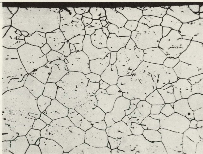
FIGURE 53 INCONEL-AS-RECEIVED AT 250 X
