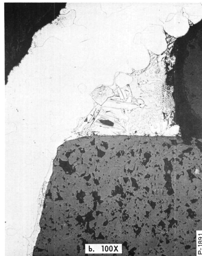
Figure 15 - Mobium-Alumina Diffusion Seal using Nickel Intermediate Material
