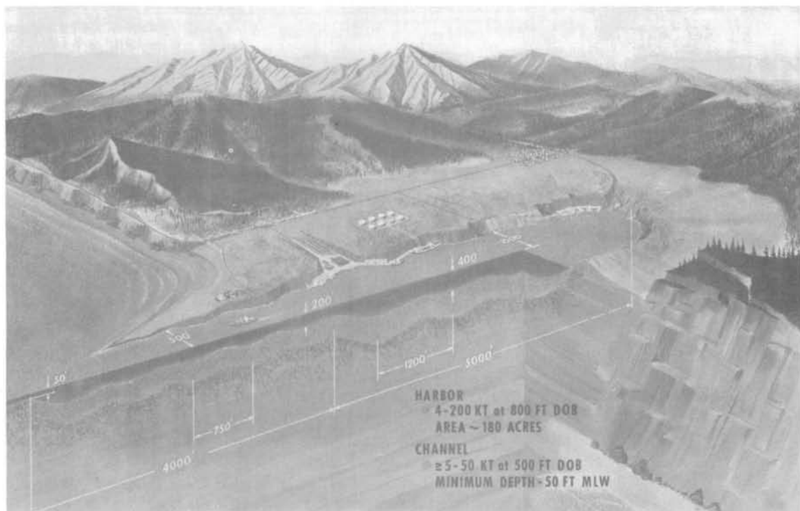
Fig. 6. Idealized plan for excavating a harbor with nuclear explosives.
