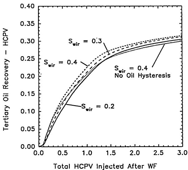
Figure 10. Effects of Water and Oil Relative Permeability Hysteresis on  $\text{CO}_2$  Flood Performance
