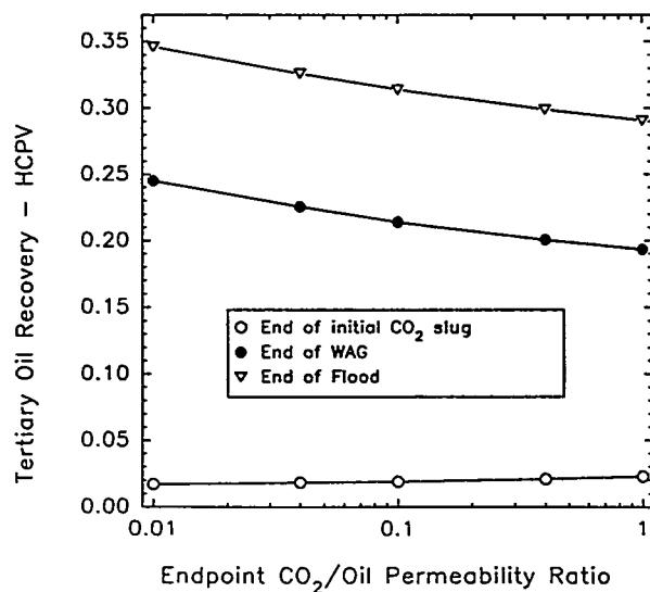
Figure 2. Effect of Endpoint CO<sub>2</sub>/Oil Relative Permeability Ratio on Tertiary Oil Recovery for the Hybrid WAG Process
