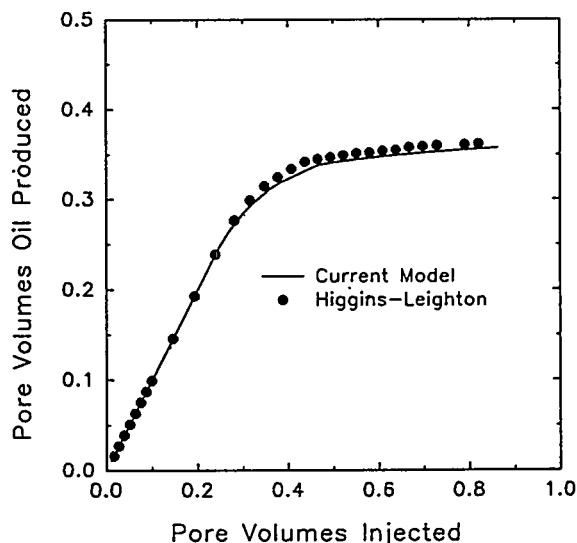
Figure A-1. Comparison of Current Model and Higgins-Leighton Method (Ref. 11) for Predicted Waterflood Performance in a Five-Spot
