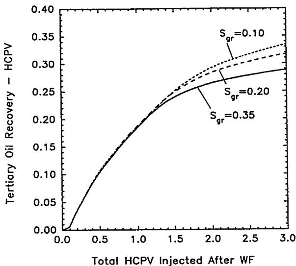
Figure 9. Effect of Residual Gas Saturation on  $\text{CO}_2$  Flood Performance
