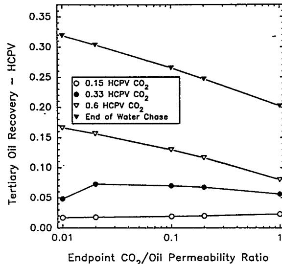
Figure 4. Effect of Endpoint CO<sub>2</sub>/Oil Relative Permeability Ratio on Tertiary Oil Recovery for the Continuous CO<sub>2</sub> Process
