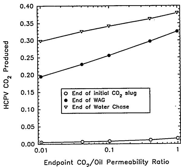
Figure 5. Effect of Endpoint  $\text{CO}_2$ /Oil Relative Permeability Ratio on  $\text{CO}_2$  Production for the Hybrid WAG Process
