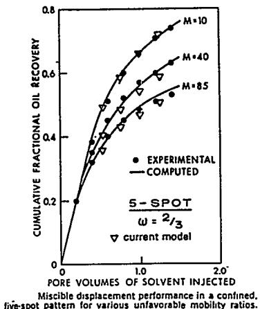
Figure A-2. Comparison of Current Model with Todd and Longstaff Results (This is Fig. 5 from Ref. 6)
