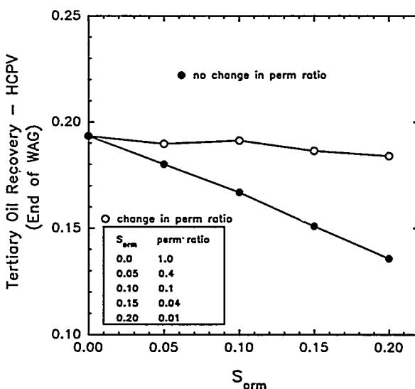
Figure 8. Effect of  $S_{\text{orm}}$  on Oil Recovery With and Without Change in  $\text{CO}_2$  Relative Permeability
