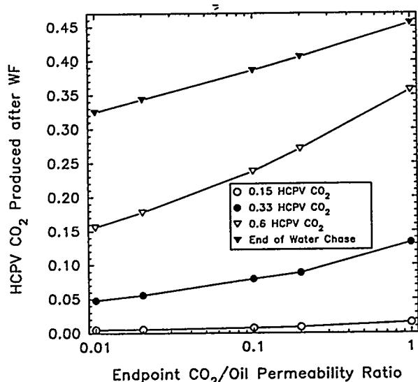
Figure 6. Effect of Endpoint  $\text{CO}_2$ /Oil Relative Permeability Ratio on  $\text{CO}_2$  Production for the Continuous  $\text{CO}_2$  Process
