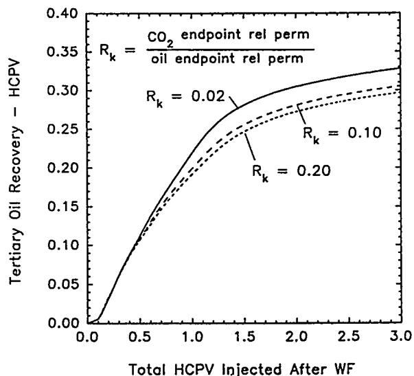
Figure 3. Impact of Endpoint CO<sub>2</sub> Relative Permeability on Oil Recovery for the Saturation Weighted Method
