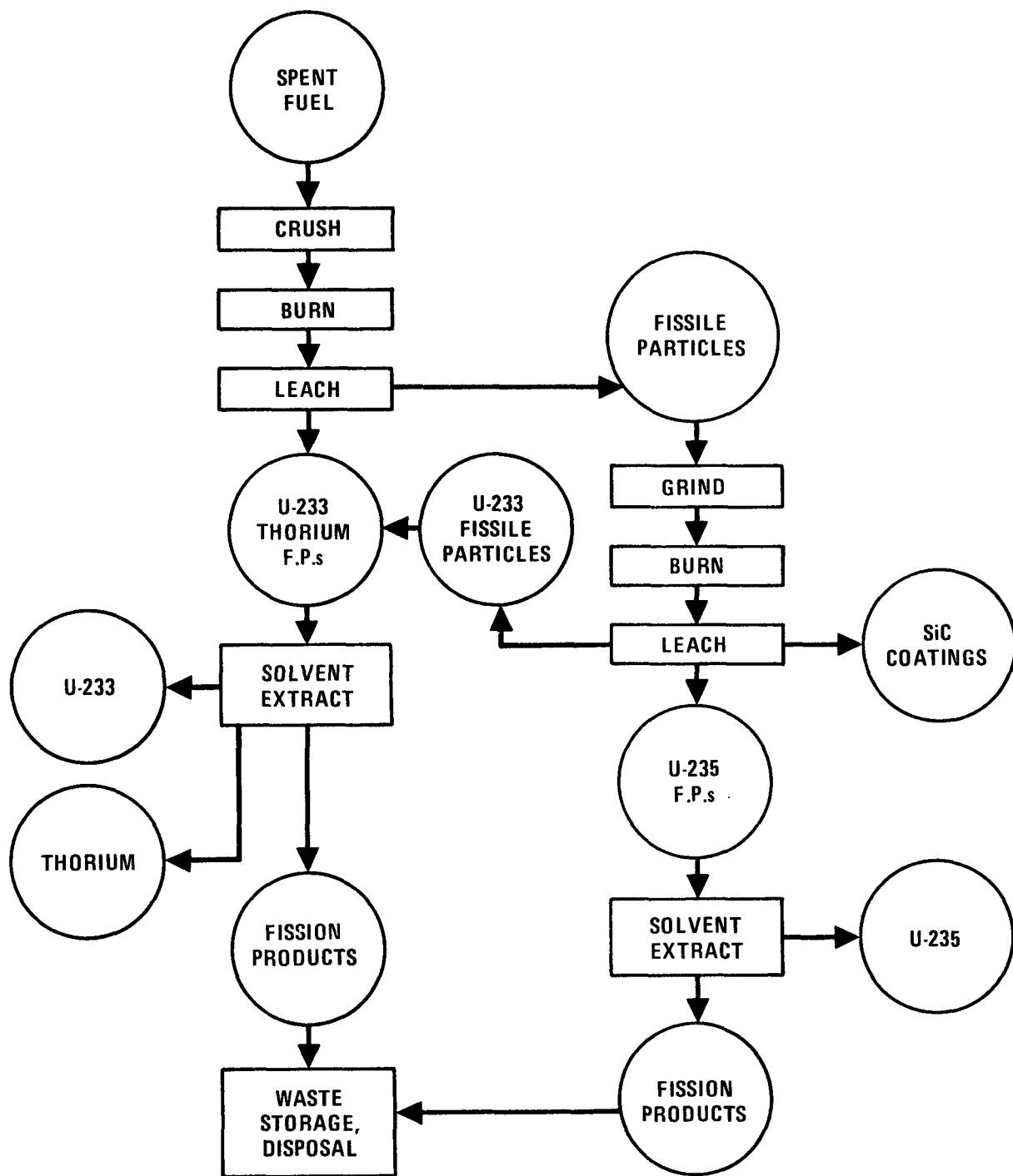
Figure 1. HTGR Fuel Processing
