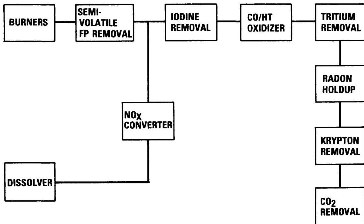
Fig. 3. Burner and Dissolver Off-Gas Treatment System
