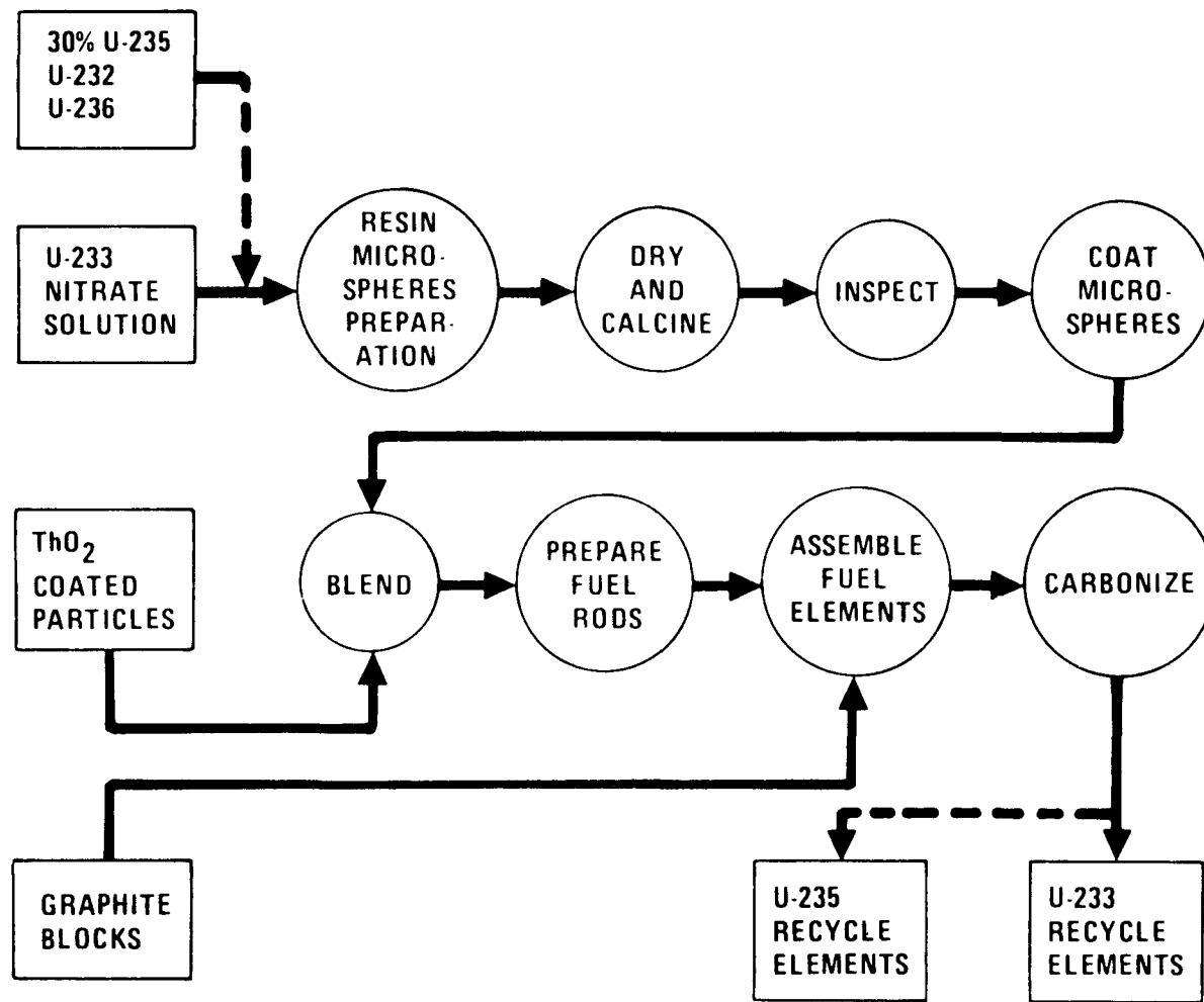
Figure 11. Simplified Refabrication Flow Diagram
