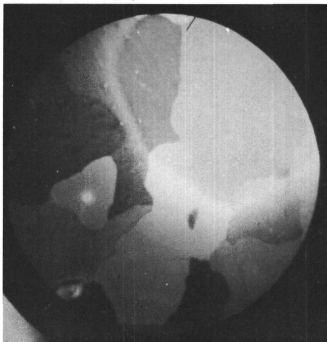
Fig. 2 Oxygen adsorption on tungsten, cloud effects
